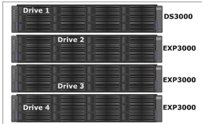
Figure 5-8 Enclosure loss protection
