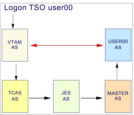
Figure 3-2 TSO/E logon process in a VTAM environment
