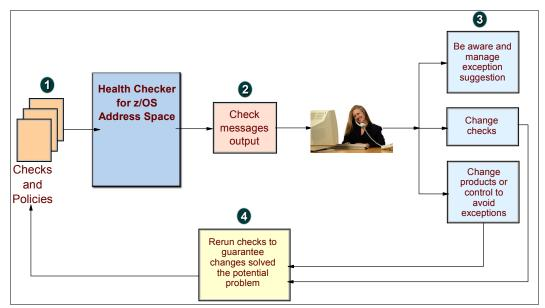
Figure 1-11 IBM Health Checker for z/OS
