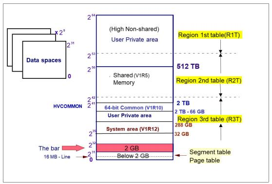
Figure 5-4 z/Architecture address space
