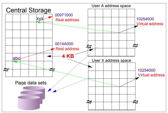
Figure 5-2 Virtual storage, auxiliary storage
