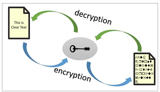
Figure 1-6 Symmetric cryptography
