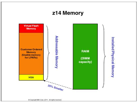
Figure 5-8 IBM Virtual Flash Memory
