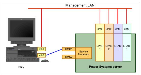
Figure 1-23 Network connections from the HMC to service processor and LPARs
