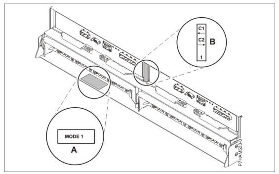
Figure 2-27 Mode sticker locations at the rear of the 5887 disk drive enclosure
