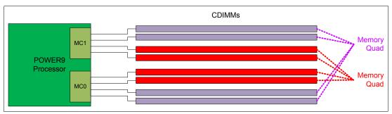
Figure 2-12 Logical diagram of a POWER9 processor and its two memory quads
