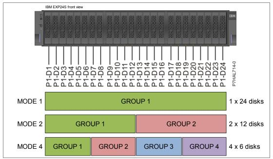
Figure 2-26 EXP24S drawer front view with location codes and disk groups
