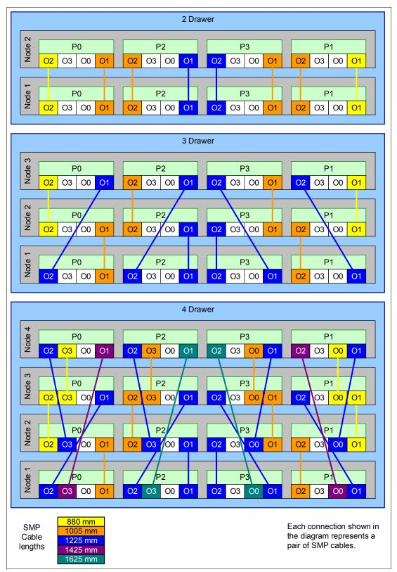
Figure 2-2 Symmetric multiprocessing cabling
