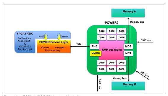
Figure 2-6 CAPI 2.0 POWER9 system block diagram
