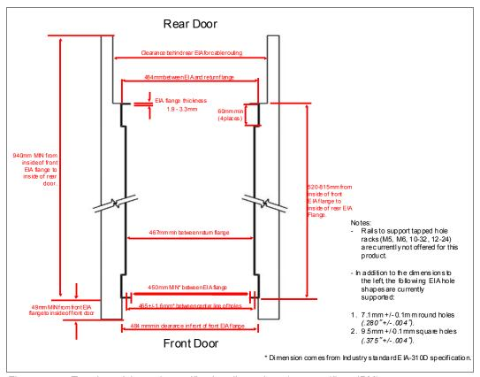
Figure 1-19 Top view of the rack specification dimensions (not specific to IBM)
