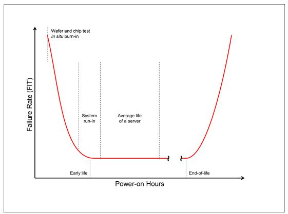
Figure 4-1 Failure rate bathtub curve
