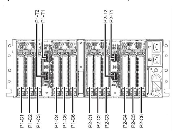
Figure 2-21 shows the connector locations for the PCIe Gen3 I/O Expansion Drawer.
