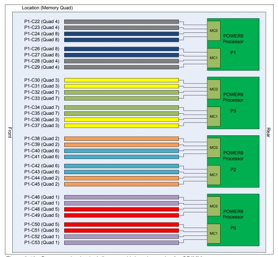
Figure 2-13 System node physical diagram with location codes for CDIMMs
