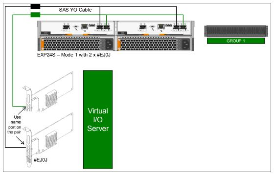
Figure 2-31 Scenario 2: Basic redundant connection
