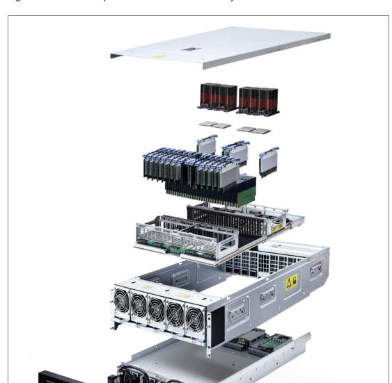
Figure 1-1 shows an exploded view of a Power E980 system node.
