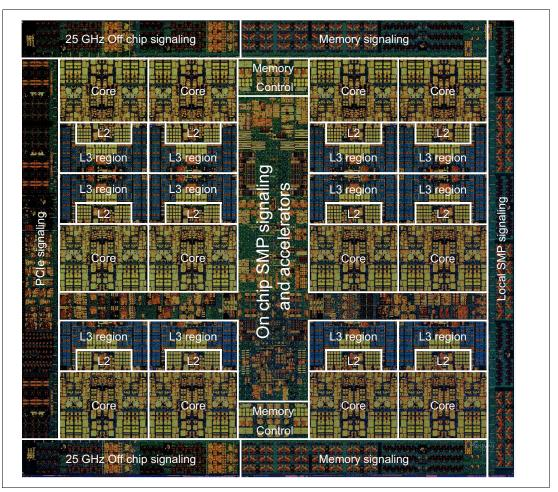
Figure 2-3 The POWER9 processor chip
