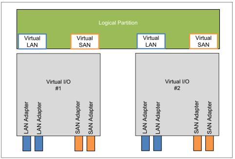
Figure 4-4 Partition with dual redundant Virtual I/O Servers
