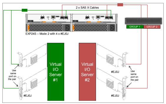
Figure 2-32 Dual Virtual I/O Servers sharing a single EXP24S drawer
