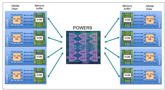
Figure 1-8 shows an example of DRAM access by using a memory buffer.
