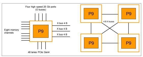
Figure 1-7 O-Bus and X-Bus fabric for Drawer to Drawer interconnect or Accelerator.
