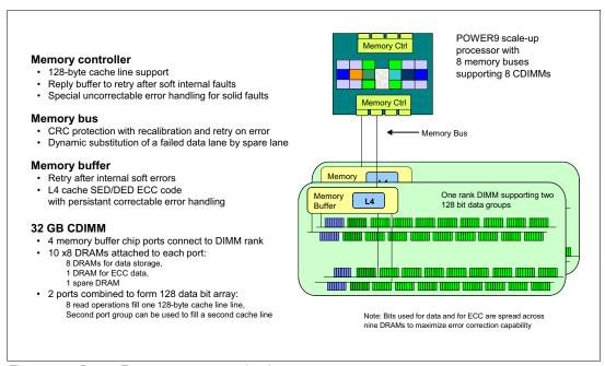
Figure 4-2 Power E980 memory protection features
