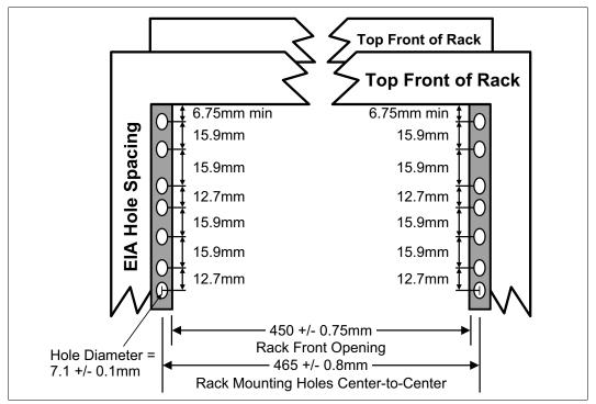
Figure 1-20 Rack specification dimensions: Top front view
