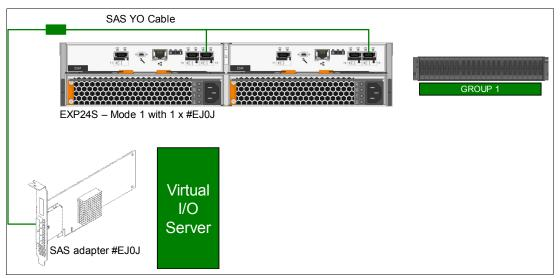
Figure 2-30 Scenario 1: Basic non-redundant connection
