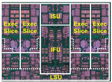
Figure 2-4 POWER9 processor chip
