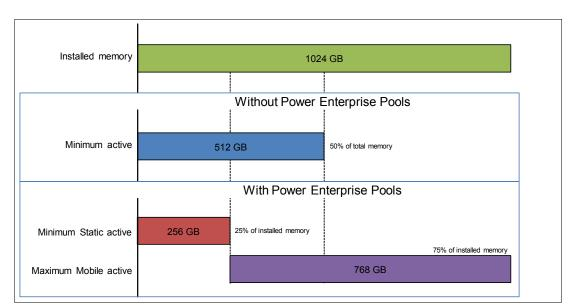
Figure 2-14 shows an example of the minimum required activations for a system with 1 TB of installed memory.
