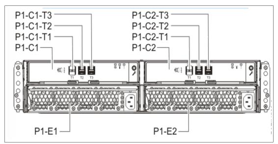
Figure 2-35 Connector locations for the EXP24SX and EXP12SX storage enclosures
