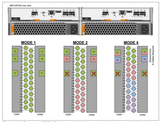
Figure 2-29 Rear view of EXP24S drawer with the 3 three modes of operation and the disks that are assigned to each port
