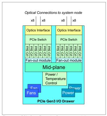
Figure 4-3 PCI3 Gen3 Expansion Drawer structural diagram
