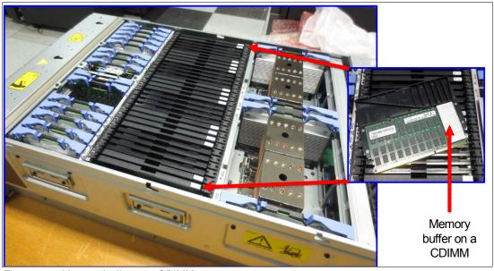
Figure 1-9 Memory buffer on a CDIMM
