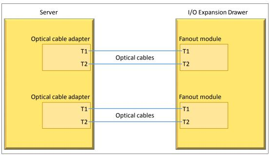
Figure 2-22 Typical optical cable connection
