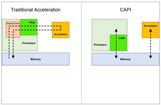
Figure 2-6 CAPI accelerator that is attached to the POWER9 processor
