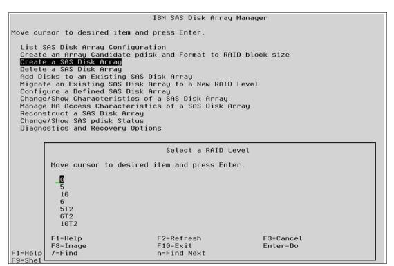
Figure 2-19 Array type selection screen on AIX RAID Manager
