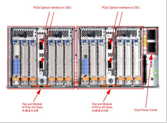
Figure 2-22 shows the back view of the PCIe Gen3 I/O expansion drawer.
