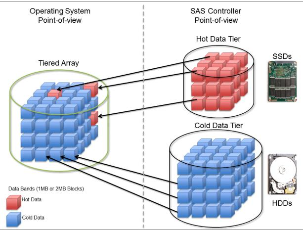
Figure 2-18 shows an Easy Tier array.
