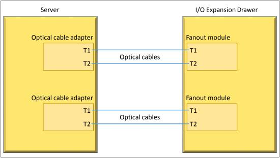
Figure 2-24 Typical optical cable connection
