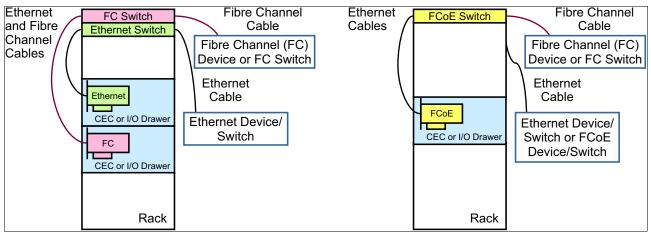
Figure 2-12 Comparison between an existing Fibre Channel and network connection and FCoE connection
