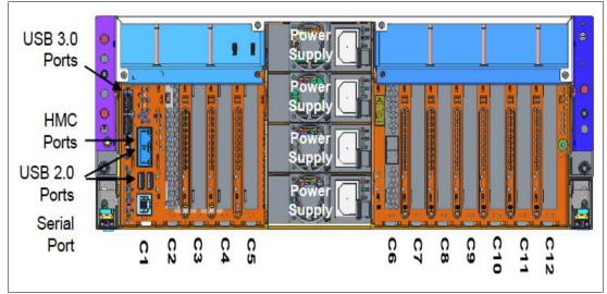
Figure 2-11 Rear view of a rack-mounted Power H924 system with PCIe slots location codes
