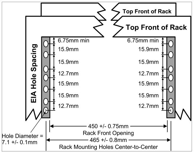
Figure 1-15 shows the top front specification dimensions.
