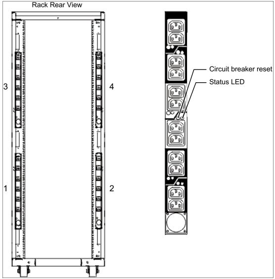
Figure 1-12 PDU placement and PDU view
