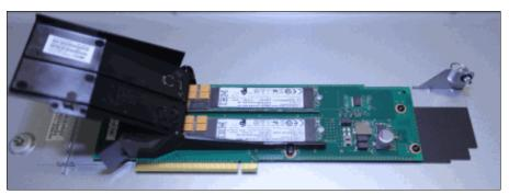
Figure 2-14 An #EC59 with the cover open showing two #EC14 modules fitted
