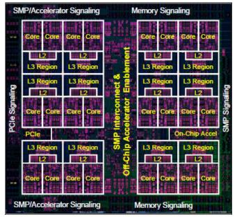
Figure 2-3 The 24-core POWER9 processor
