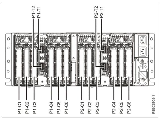
Figure 2-23 Connector locations for the PCIe Gen3 I/O expansion drawer
