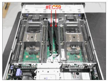
Figure 2-13 Two #EC59 components in a Power H922 server
