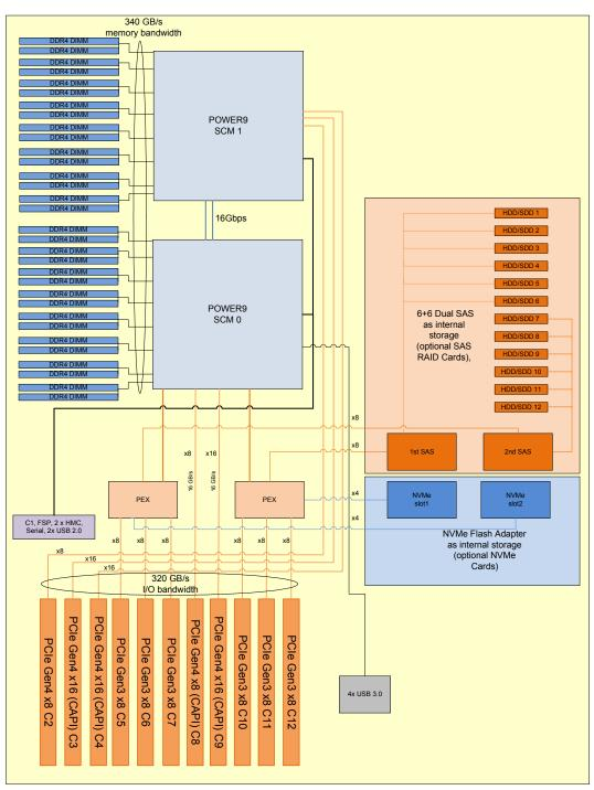
Figure 2-1 The IBM Power H924 logical system diagram
