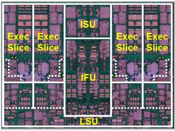
Figure 2-4 POWER9 processor core
