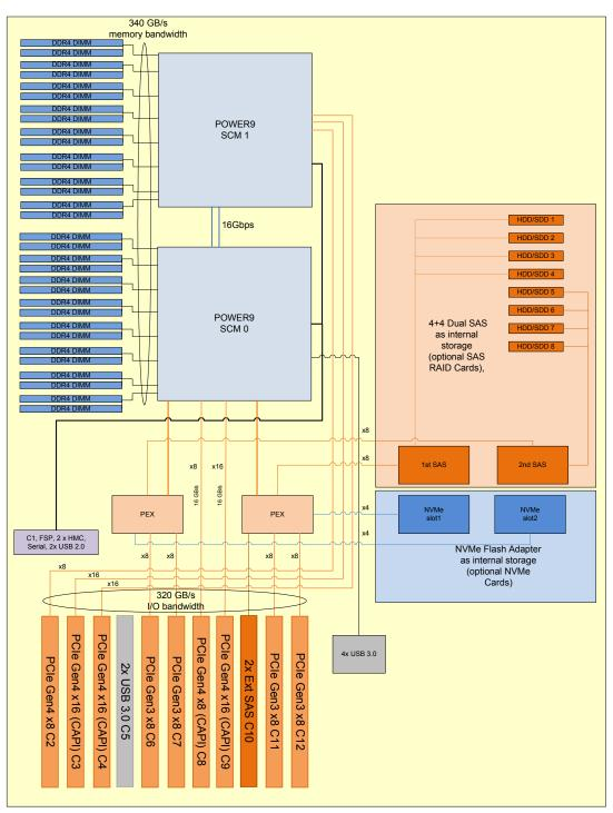
Figure 2-2 The IBM Power H922 logical system diagram
