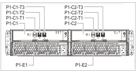
Figure 2-25 Connector locations for the EXP24SX and EXP12SX storage enclosures
