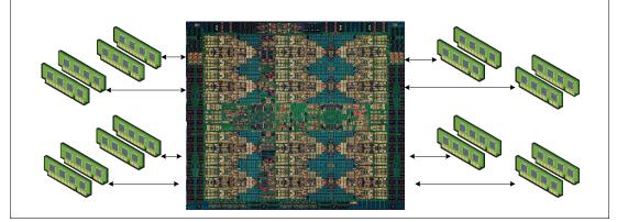
Figure 2-5 Overview of POWER9 direct-attached memory
