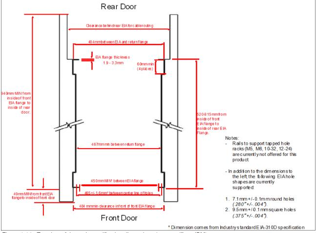
Figure 1-14 is a top view that shows the specification dimensions.
