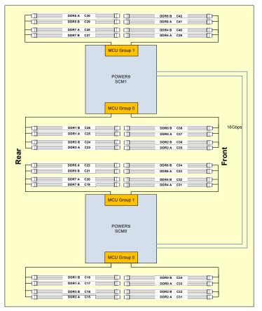
Figure 2-7 shows the physical memory DIMM topology for the Power H922 and the Power H924 servers.
