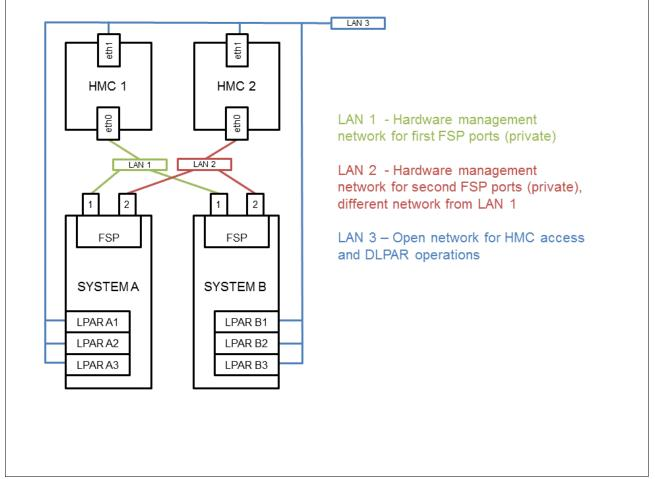
Figure 1-18 Highly available HMC networking example.
