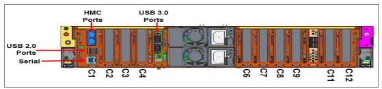
Figure 2-10 Rear view of a rack-mounted Power H922 system with PCIe slots location codes
