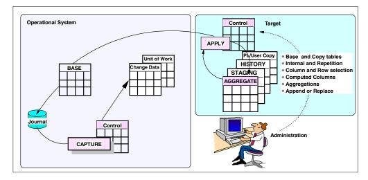
Figure 27. The DataPropagator/400 Apply process
