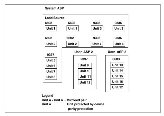
Figure 43. Mirrored protection in the system ASP and device parity protection in the user ASPs
