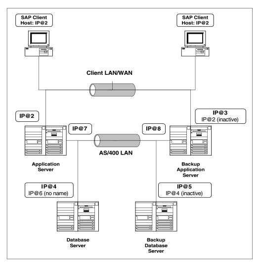
Figure 19. Three-tiered configuration: IP assignments
