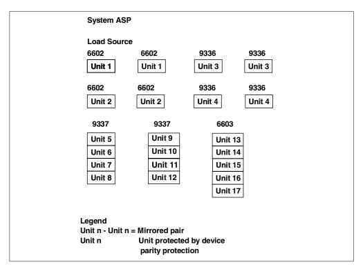
Figure 42. Mirrored protection and device parity protection to protect the system ASP
