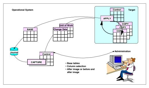
Figure 26. The DataPropagator/400 Capture process
