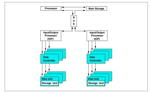
Figure 38. Components used for data transfer
