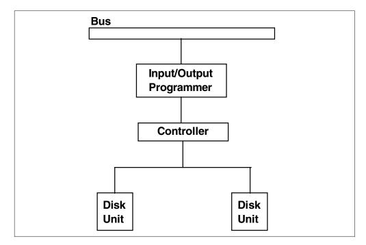
Figure 7. Disk unit level protection
