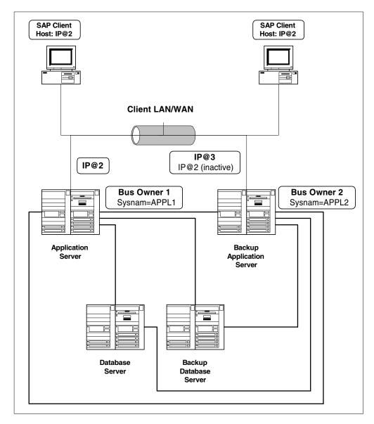
Figure 18. Three-tiered configuration: OptiConnect assignments
