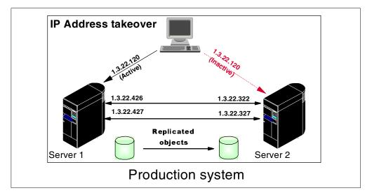
Figure 17. IP address takeover between two systems in a cluster
