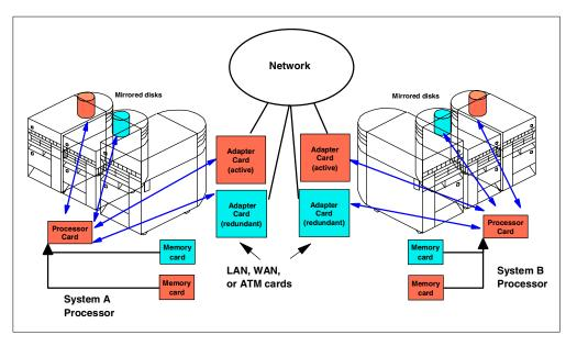
Figure 15. Redundant network connections
