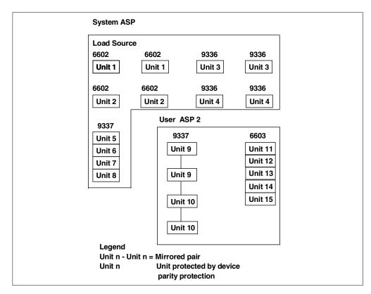
Figure 44. Mirrored protection and device parity protection in all ASPs
