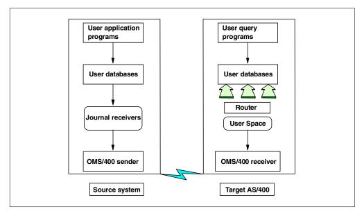
Figure 33. Object Mirroring System/400
