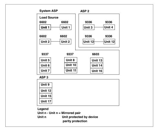
Figure 41. Different protection for multiple ASPs
