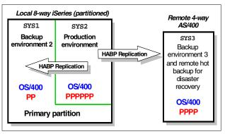
The highest level of availability is obtained with two separate servers. Figure 13 shows that, with clustering active, data is replicated to both the local backup server and the remote server. In the event of a disaster (or the need for the entire local hardware to be powered off), the remote backup server is
