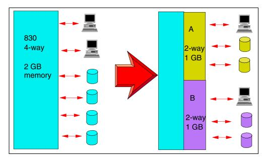
Figure 22. Example LPAR configuration
