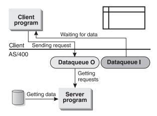
In the third state, the server program fills data queue 'I'. The client program becomes active and puts the data into the subfile. After this, the program returns to its initial state and the process starts again.
