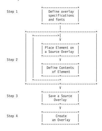
Figure 13. Overview of Overlay Utility Operation
