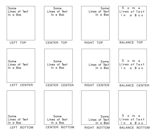
Figure 25. Example of Center-and-Trim Mapping
