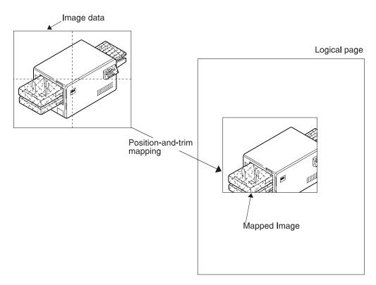
Figure 19. Position-and-trim mapping
