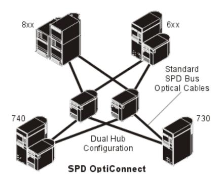
SPD OptiConnect is a combination of hardware and software that allows you to connect multiple high-end iSeries servers through a high-speed, fiber-optic bus. This combination of optical bus speeds and efficient software makes OptiConnect a viable solution, providing multiple routes to the database. You can run both APPC or TCP/IP communications protocols over OptiConnect. TCP/IP support was added to OptiConnect beginning with OS/400 or i5/OS V4R4.
