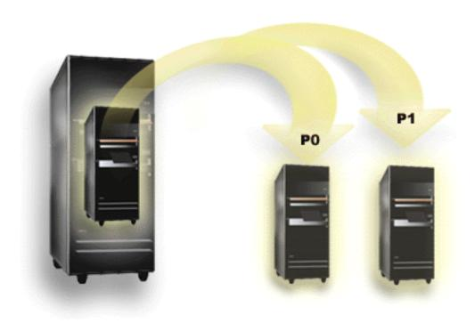
Logical partitioning is the ability to make an iSeries server run as if it were two or more independent servers. Each logical partition operates as an independent logical server. However, each partition shares a few physical system attributes such as the system serial number, system model, and processor feature code. All other system attributes may vary among partitions.
