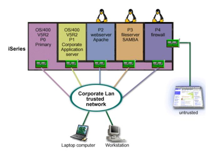
You had the hardware resources on your server to create another guest partition using iSeries Navigator. You installed Linux in partition P4. The firewall is built into the kernel that you are using. Your Linux firewall partition owns a directly attached LAN adapter that protects the entire system from untrusted
