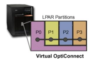
Virtual OptiConnect emulates external OptiConnect hardware by providing a virtual bus between logical partitions. You can use virtual OptiConnect without any additional hardware requirements. To use virtual OptiConnect, you only need to purchase OptiConnect for i5/OS (a priced optional feature).
