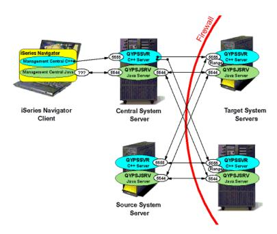
Figure 11. Endpoint Systems protected by a firewall
