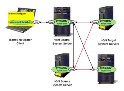
Figure 5. Connections for Java extensions for Management Central (BDT connections in Red)
