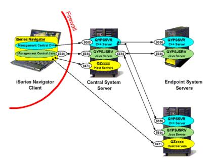
Figure 9. Graphical Client protected by a firewall
