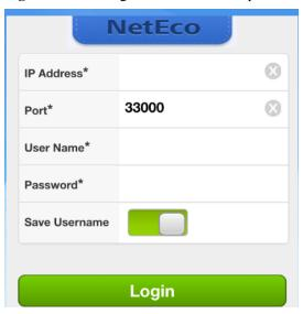
Figure 5-87 Setting the IP address and port number of the server
