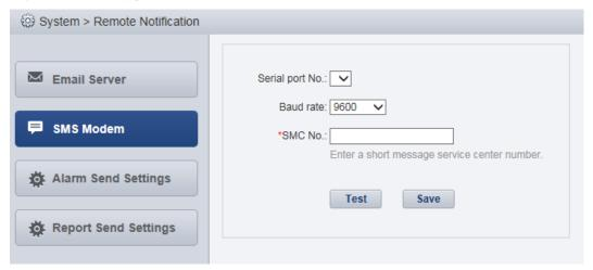
**Step 3** Setting parameters for SMS modem by referring to **Table 5-30**.
