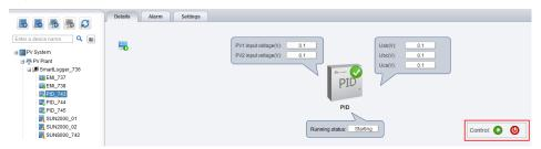
**Step 4** Issue the control commands to the PID device according to **Table 5-17**.
