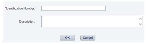
**Step 3** Enter the identification number of the mobile terminal that is allowed to access the NetEco, set **Description**, and click **OK**.
