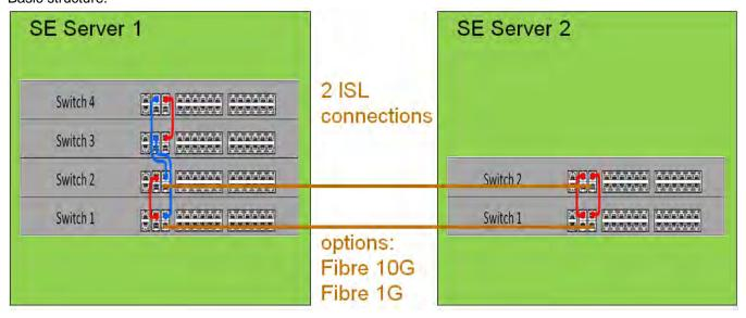
The private management and data networks configured on the ISL connections are virtual LANs. If an ISL connection is directed through the customer's infrastructure then the VLAN IDs 600..608 (for private management networks) and 800..899 (for private data networks) must be provided. Other connections are possible, but they must be verified in the course of a special release or be implemented as a customer project.
