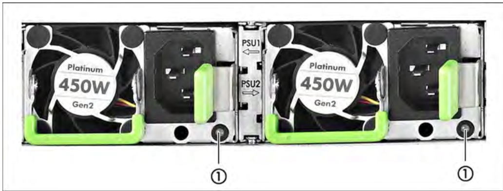
Figure 29: Indicator on hot-plug power supply unit
