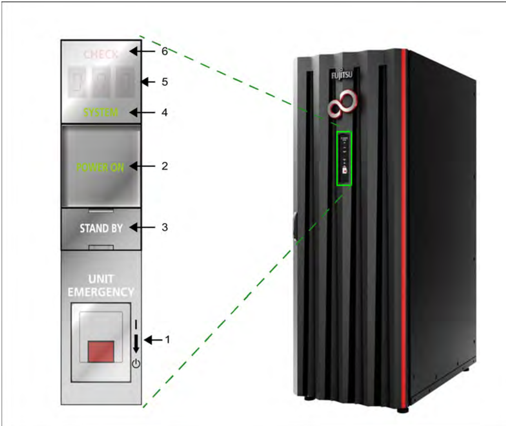
Figure 12: Control panel on the rack of the SE700 / SE700B and SE500 / SE500B
