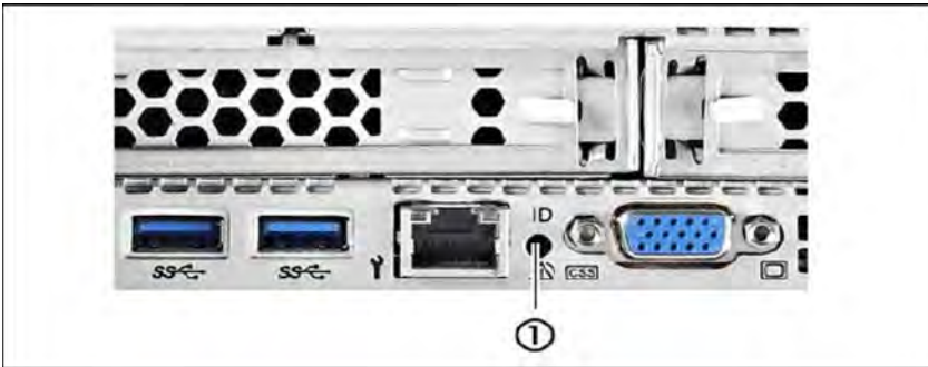
Figure 24: ID/CSS/Global error indicator (MU M2)
