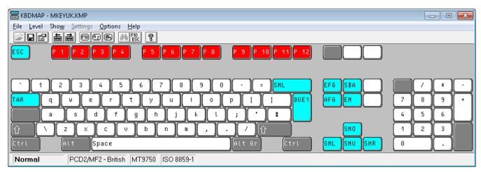
The MT9750 keyboard mapping program supports MF2 keyboards and the bimodal library keyboard. Operation of the keyboard mapping program depends on the connected keyboard and the resulting keyboard layout.
