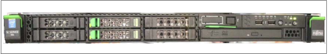
Figure 8: Management Unit (MU) - front of a MU M1
