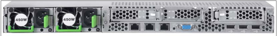
Figure 13: Management Unit (MU) - rear of a MU M1
