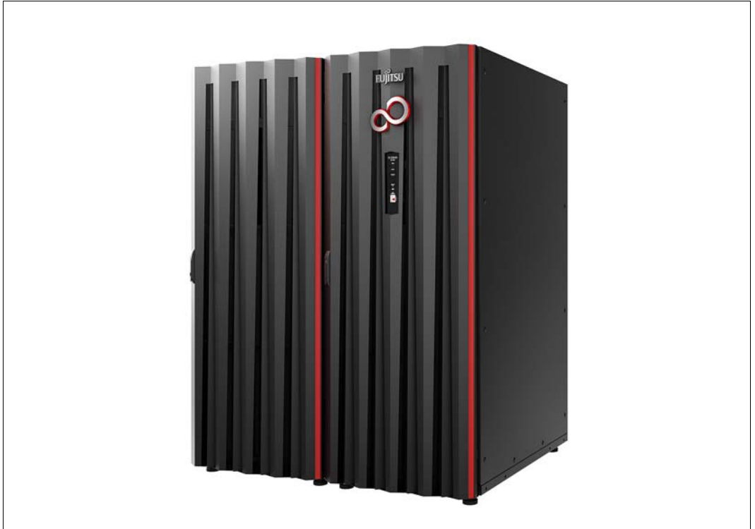
Figure 5: SE server with an extension rack (e.g. SE700 and SE700B)
