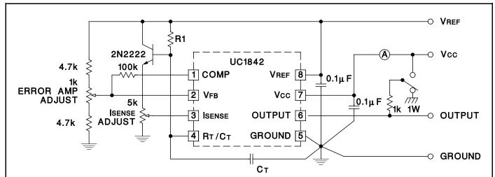
High peak currents associated with capacitive loads necessitate careful grounding techniques. Timing and bypass capacitors should be connected close to pin 5 in a single point
