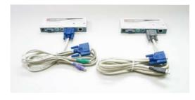
The KVM Extender consists of a Computer Unit and a Station Unit that enables you to locate a keyboard/monitor/mouse setup up to 150 meters away from a computer or KVM switch using an inexpensive Category 5 UTP (unshielded twisted pair) cable. This provides a convenient way to remotely access a computer located in a secure or not easily accessible environment.
