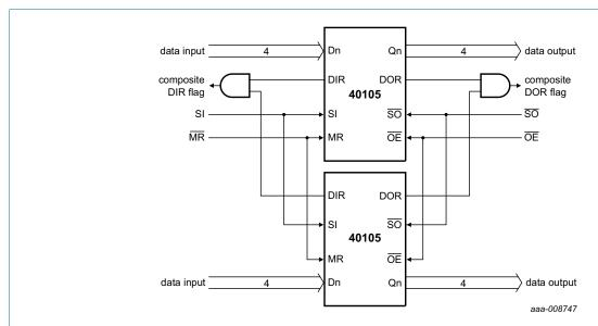
The 74HC40105; 74HCT40105 is easily expanded to increase word length. Composite DIR and DOR flags are formed with the addition of an AND gate. The basic operation and timing are identical to a single FIFO, except for an added gate delay on the flags.
