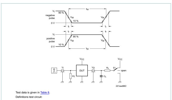
$R_T$  = Termination resistance should be equal to output impedance  $Z_o$  of the pulse generator.
