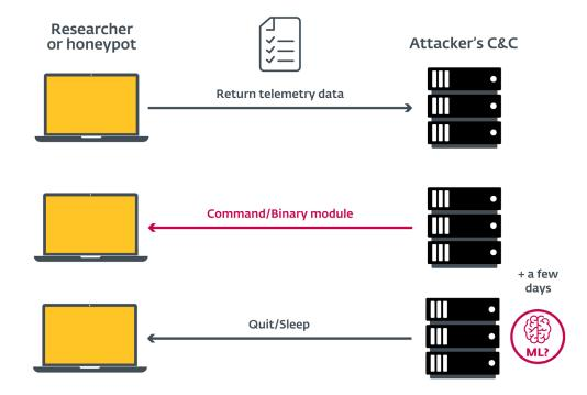
Figure 13 // Researcher machine (honeypot) reports enhanced artificial telemetry data to the attacker's C&C, receives command or binary module. After few days Emotet switches again to quit/sleep command.
