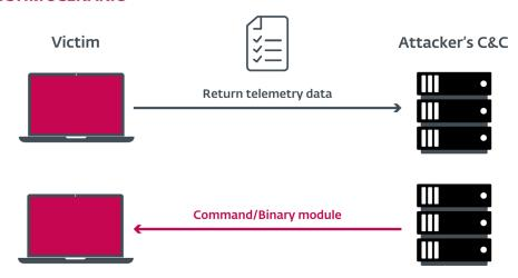
Figure 11 // Compromised victim machine reports genuine telemetry data to the attacker's C&C, receives command or binary module.
