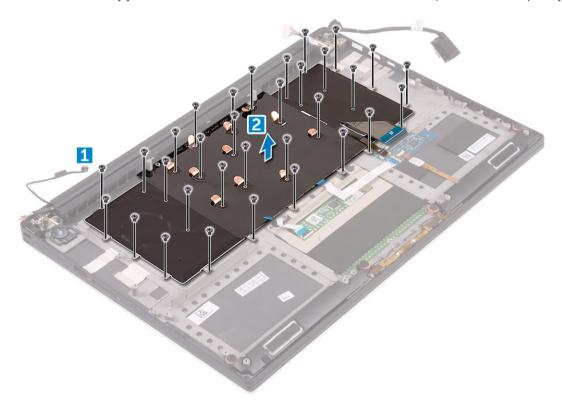
5 Lift and remove the keyboard from the computer.
