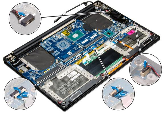
5 Perform the following steps to remove the system board from the computer:
