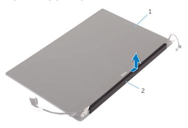
Figure 7. Removing the antenna cover
