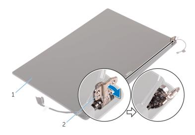
Figure 6. Turning the display hinge
