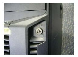
Figure 13. Bezel Lock in Front Bezel
