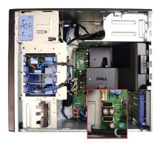
Figure 17. Internal USB Connectors
