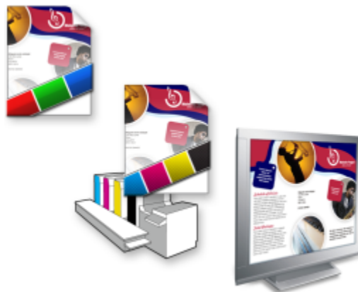
Top left: An RGB color profile is assigned to the document. Middle and right: Assigning a specific CMYK profile allows an on-screen simulation of the printed output.
