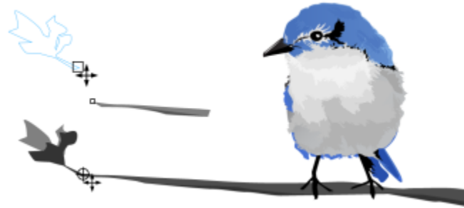
The pointer was snapped to an end node of the leaf (top), and then the leaf was dragged to snap to the end node of the branch (bottom).
