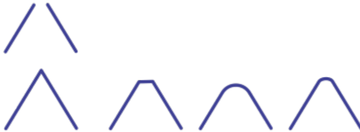
The lines in the upper-left corner were joined by using different modes. Modes from left to right: Extend, Chamfer, Fillet, and Bézier Curve.
