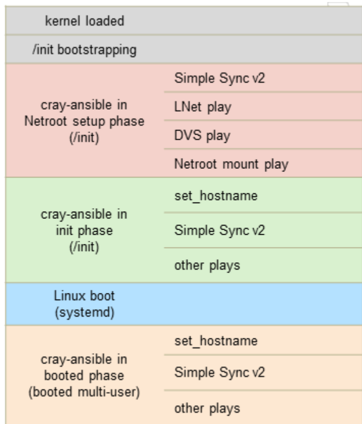
Figure 10. Node Image at Boot Time using Netroot
