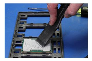
**12.** Clean the thermal grease off the heatsink using a plastic scrapper and isopropyl alcohol.
