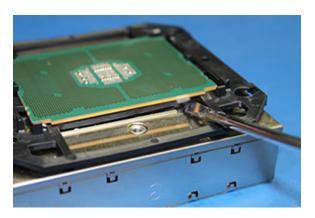
**10.** Hold the processor on either side with two fingers and bend back either the top or bottom of the processor tray to release the processor from the retaining clips.
