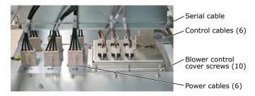
**6.** Remove the 10IP Torx+ screws (4) that attach the blower control assembly to the PDU and remove the assembly.
