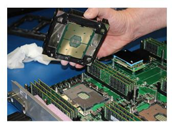
**8.** Tighten the four T15 screws in the correct order and torque to 9 in-lbs.
