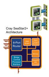
Designed for scalable MPI computing, the Cray SeaStar2+ chip combines communications processing and high-speed routing on a single device. Each communications chip is composed of a HyperTransport™ link, a Direct Memory Access (DMA) engine, a communications and management processor, a high-speed interconnect router, and a service port.
