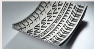
← Outillage de pneu [Acier Maraging]. AUTOMOBILE
