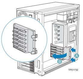
Figure 54: Removing PCI Card Guide
