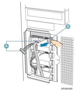
Figure 67: Preparing Fixed Hard Drive for Removal
