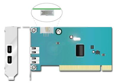
Figure 13: IEEE 1394 Controller Card (Low profile bracket shown)
