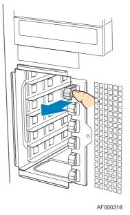
Figure 56: Unlatching Drive Latch
