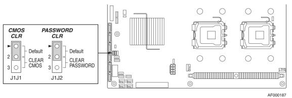
Figure 8: CMOS Clear Jumper
