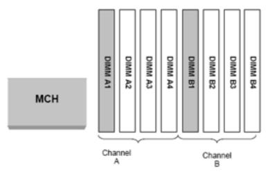
Figure 12: Two DIMM Memory Configuration
