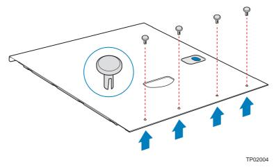
Figure 31: Removing the Plastic Plugs from the Top Side Cover
