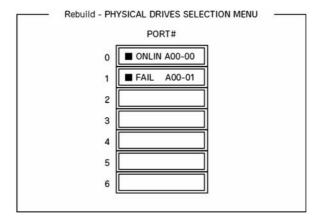
Figure 41: Rebuild – Physical Drives Selection Menu
