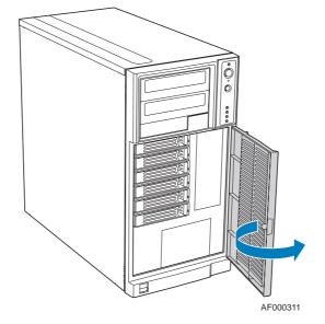
Figure 70: Opening the Drive Bay Access Door
