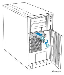
Figure 71: Removing the Drive Carrier from the Hot Swap Drive Cage
