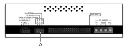
Figure 106: Connectors on the Back of an Optical Drive (example)
