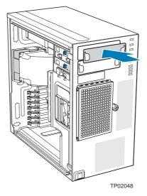
Figure 51: Installing 5.25-in Drive EMI Shield
