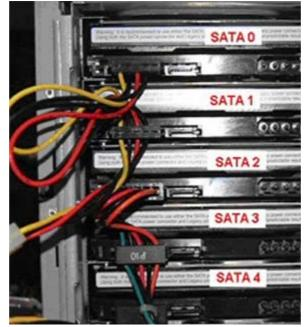
Figure 61: Using a SATA/MOLEX Power Adapter
