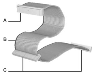
Figure 96: Three-connector IDE Cable
