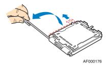
Figure 83: Lifting the Processor Lever
