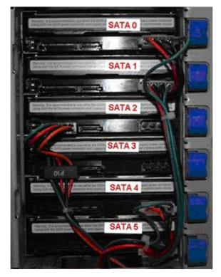
Figure 62: Using a MOLEX Power Port
