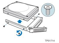
Figure 72: Removing the Hard Drive from the Drive Carrier
