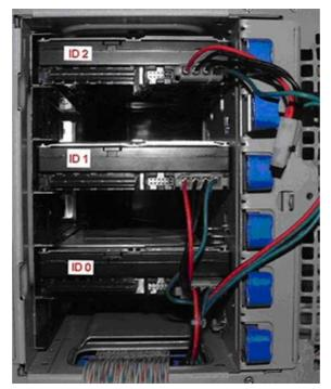
Figure 59: Three SCSI Hard Disk Drives Installed
