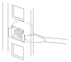
Figure 30: Inserting a caged nut
