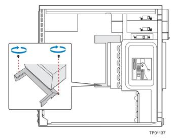
Figure 88: Installing Large Processor (Part A) Air Duct
