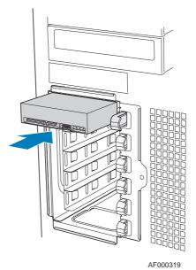
Figure 57: Inserting Hard Drive into Drive Cage
