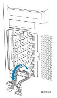
Figure 55: Routing Hard Drive Power Cables
