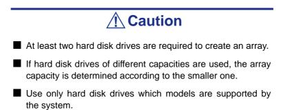
■ The hard disk drive which has been configured as an array disk drive cannot be selected.
