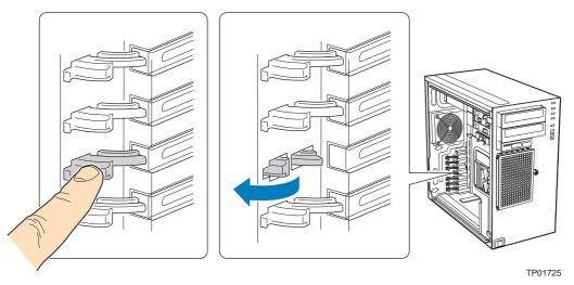
Figure 93: Opening the PCI Add-in Card Retention Device
