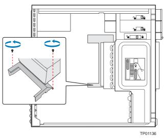
*Figure 82: Removing Large Processor (Part A) Air Duct* Save the screws. You will need them to re-install the processor air duct.
