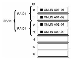
Figure 40: Spanning of RAID1
