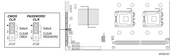
Figure 6: CMOS and Password Clear Jumpers
