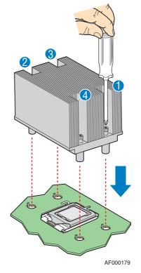
Figure 87: Installing the Heat Sink
