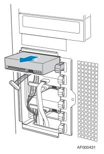
Figure 68: Removing Fixed Hard Drive from Drive Bay
