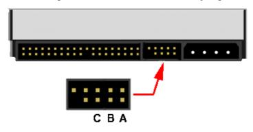
Figure 108: Connectors on the Back of a Tape Drive (example)
