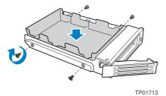
Figure 74: Installing the Plastic Retention Device in the Drive Carrier
