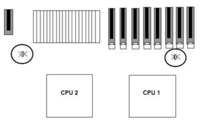
Figure 111: CPU Fault LEDs
