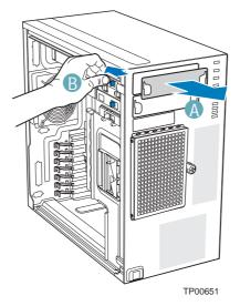
Figure 48: Removing 5.25-inch Drive EMI Shield
