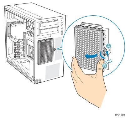
Figure 53: Removing Drive Cage EMI Shield from Chassis
