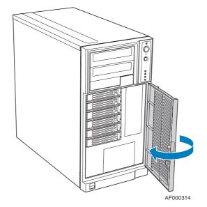
Figure 76: Closing the Drive Bay Access Door
