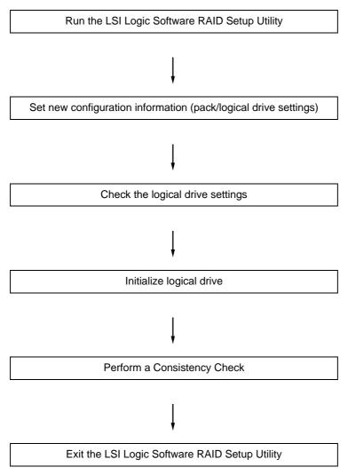
1. Run the LSI Logic Software RAID Setup Utility.
