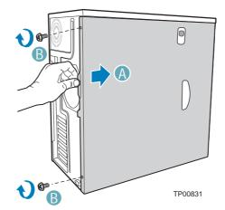
Figure 45: Replacing the left side cover A: sliding the left side cover forward B: screws
