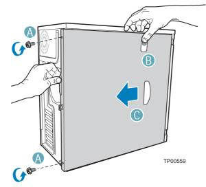
Figure 44: Removing the cover
