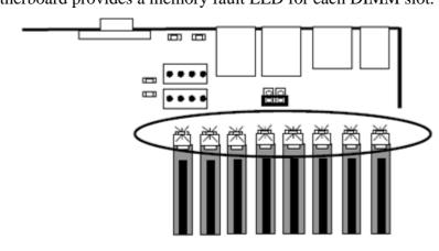
The motherboard provides a memory fault LED for each DIMM slot.
