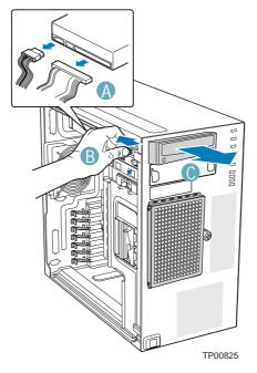
Figure 50: Removing an Optical Disc Drive
