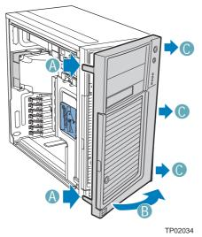
Figure 46: Removing the Front Panel
