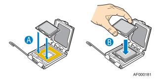
Figure 86: Installing the Processor
