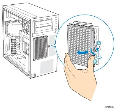
Figure 66: Removing the Drive Cage EMI Shield
