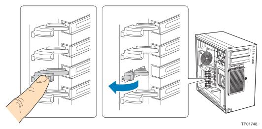
Figure 90: Opening the PCI Add-in Card Retention Device
