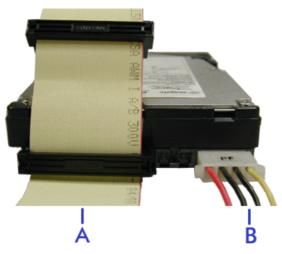
Figure 99: Cabling a SCSI Hard Disk Drive
