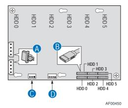
Figure 78: SAS/SATA Backplane Cable connectors (Backplane without expander shown)
