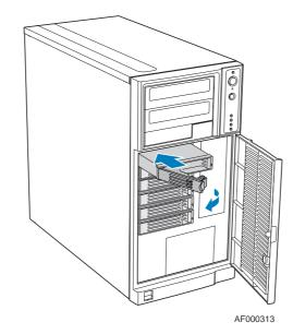
*Notes*: For proper airflow, the drive carrier must be replaced in the chassis, even if no hard drive is installed in it.
