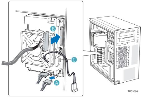
Figure 81: Cabling the SCSI Hot Swap Drive Cage
