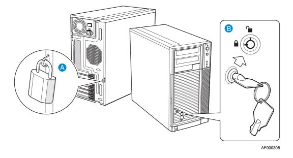
Figure 109: WA2500/SA2500 Security Features A: Padlock loop B: Two-position mechanical lock
