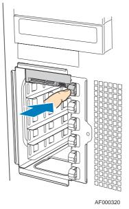
Figure 58: Latching Drive Latch
