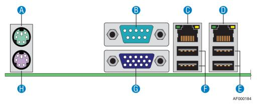
Figure 10: Back Panel Connectors
