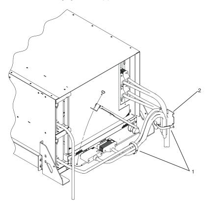
Securing Drawer Cables: Route the cables over the cable guides (2), and secure the cables with Velcro strips (1). Leave a loop that is large enough so that the drawer can be pulled out the back.
