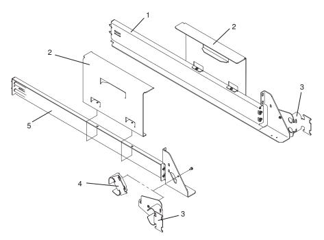
3. Install the rails in the rack unit. As you install the right rail into the rack, install the drawer latch reset bracket above the right rail.
