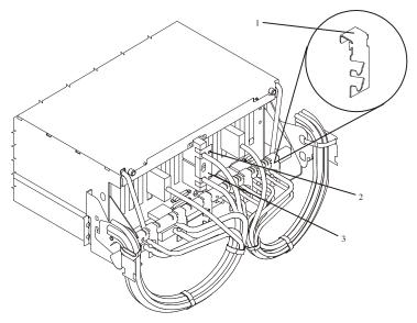
**CEC Drawer Cables**: Route the CEC drawer cables toward the right rack rail, and secure the cables with Velcro strips (1).
