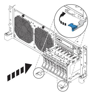
Figure 50. Replacing the disk drive cage
