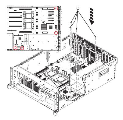
Figure 42. Installing the system backplane
