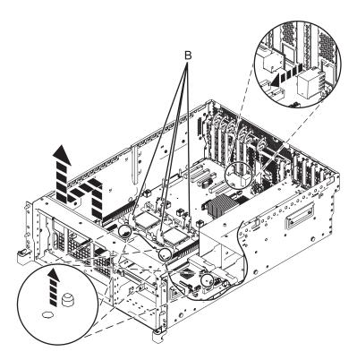
Figure 40. Removing the system backplane
