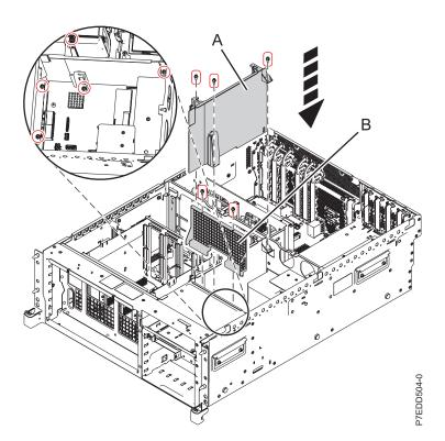
Figure 47. Replacing the disk-drive cage shield in the 02E/4C, 02E/4D, 05E/6C, or 05E/6D
