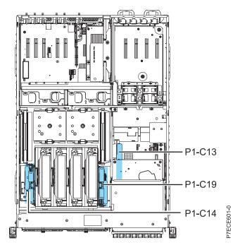
Figure 5. Slot location for the RAID enablement card, the RAID/cache storage controller, and the cache battery card
