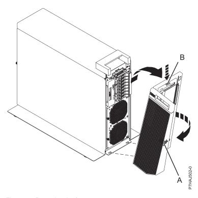
Figure 57. Removing the front cover
