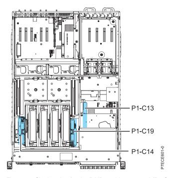
Figure 10. Slot location for the RAID enablement card (P1-C13)
