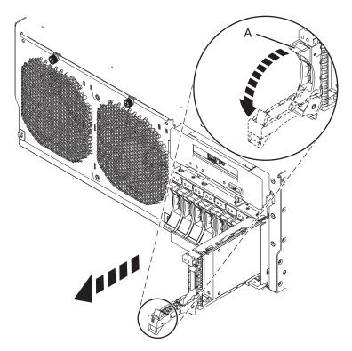
Figure 22. Removing the disk drive from the backplane
