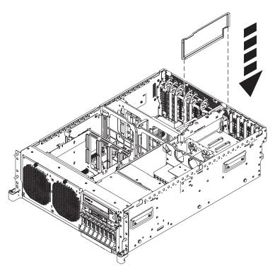
Figure 49. Replacing the PCI riser air divider
