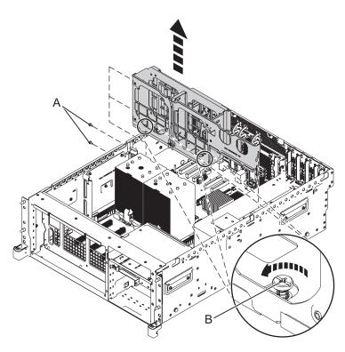
Figure 38. Remove the middle fan cage
