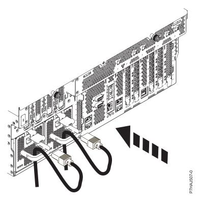
Figure 73. Connecting the power cords
