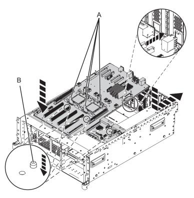
Figure 41. Installing the system backplane in the 02E/4B or 05F/6B
