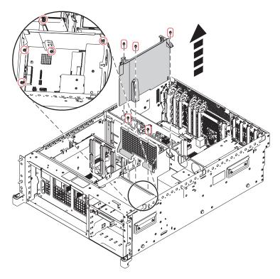
Figure 35. Removing the disk-drive cage shield from the 02E/4C, 02E/4D, 05E/6C, or 05E/6D
