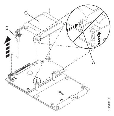
Figure 18. Removing the cache battery
