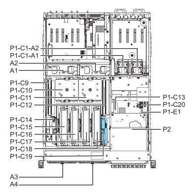
Figure 1. Slot locations of RAID-10 storage controller (P1-C19) for the 02E/4B or 05F/6B
