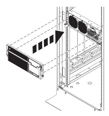
Figure 58. Removing the front cover
