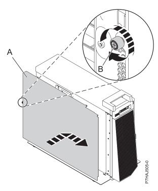
Figure 66. Installing the outside service access cover
