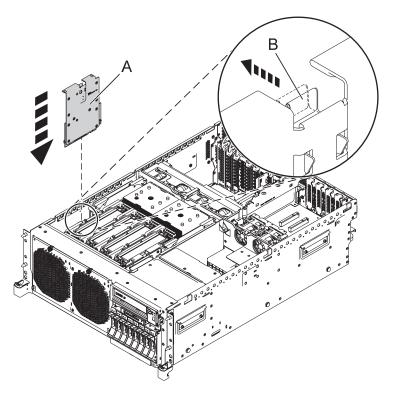
Figure 17. Installing the cache battery card
