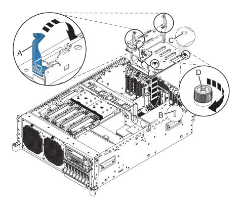
Figure 48. Replacing the PCI riser
