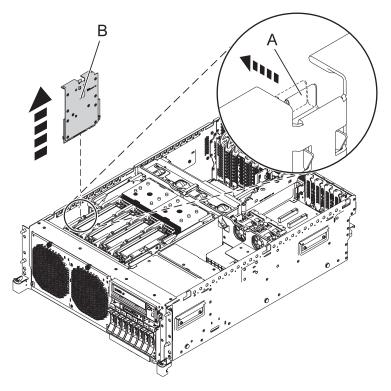
Figure 16. Removing the cache battery card
