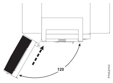
Figure 60. Installing the front door
