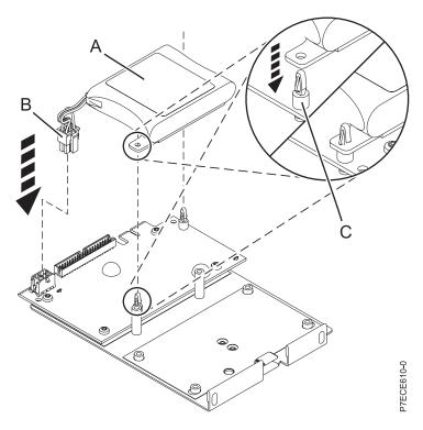
Figure 19. Replacing the cache battery
