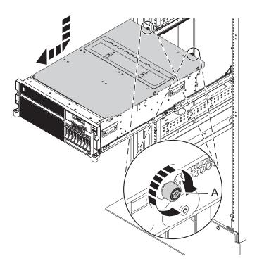
Figure 64. Installing the service access cover
