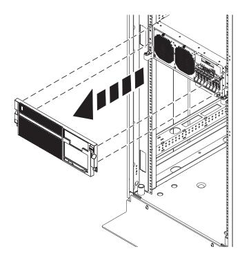
Figure 56. Removing the front cover
