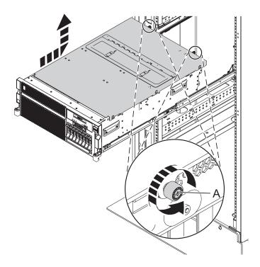
Figure 61. Removing the service access cover
