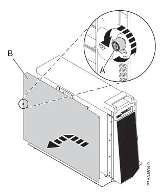
Figure 62. Installing the outside service access cover
