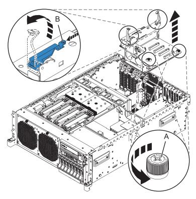
Figure 33. Removing the PCI riser
