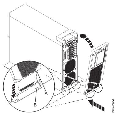
Figure 59. Installing the front cover
