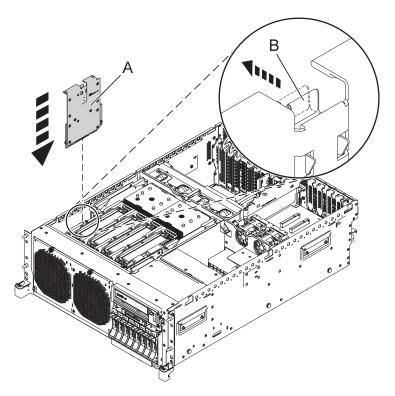
Figure 9. Rack-mounted model RAID cache battery card replacement
