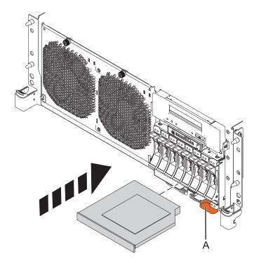
Figure 29. Installing the media device
