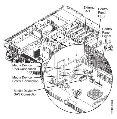
Figure 30. Disconnecting the internal cables
