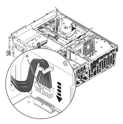
Figure 44. Connecting the front fan cable
