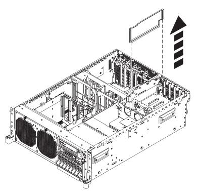
Figure 32. Removing the PCI riser air divider
