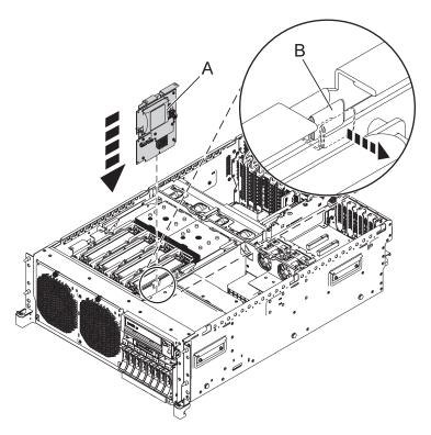
Figure 8. Rack-mounted model RAID/cache storage controller replacement
