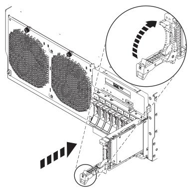
Figure 28. Installing the backplane disk drives
