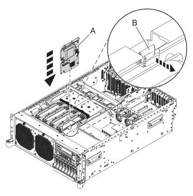
Figure 4. Rack-mounted model RAID-10 storage controller replacement
