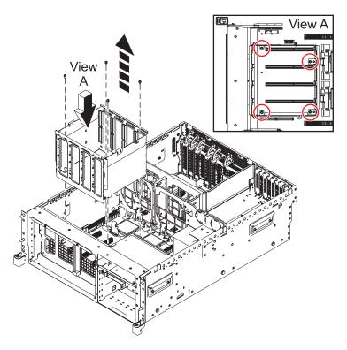
Figure 36. Removing the DIMM cage
