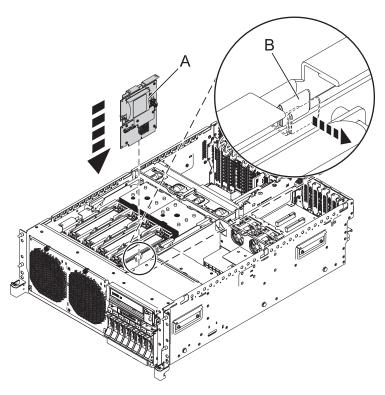
Figure 2. Rack-mounted model RAID-10 storage controller replacement
