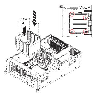
Figure 45. Replacing the DIMM cage
