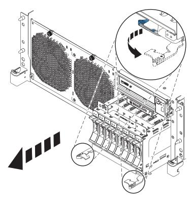
Figure 31. Removing the disk drive cage
