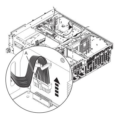
Figure 37. Disconnecting the front fan cable
