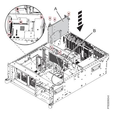
Figure 46. Replacing the disk-drive cage shield in the 02E/4B or 05F/6B
