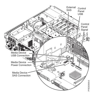
Figure 51. Connecting the internal cables
