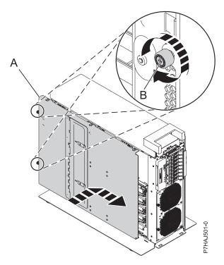
Figure 65. Installing the inside service access cover
