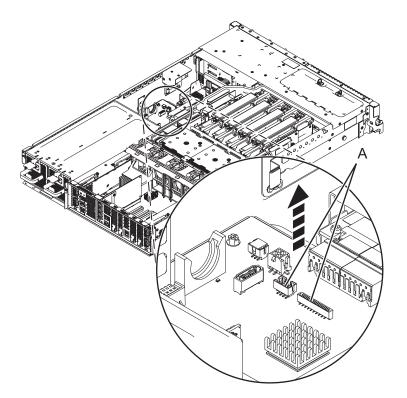
Figure 38. Disconnecting the operator panel cable
