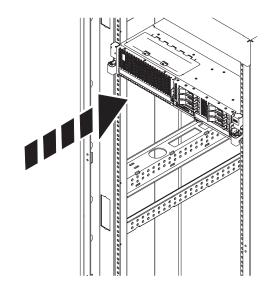
Figure 70. Placing the system in the operating position
