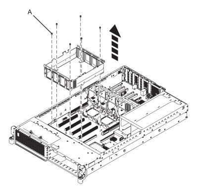
Figure 44. Removing the DIMM cage
