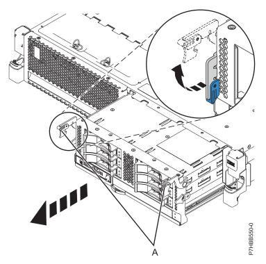
Figure 31. Removing the backplane populated with disk drives
