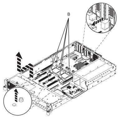
Figure 48. Removing the system backplane from the 31E/2B
