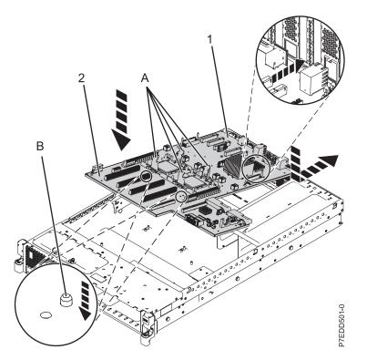
Figure 50. Replacing the system backplane in the 31E/2B
