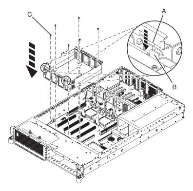
Figure 55. Replacing the DIMM cage
