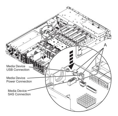
Figure 59. Connecting the media device cables
