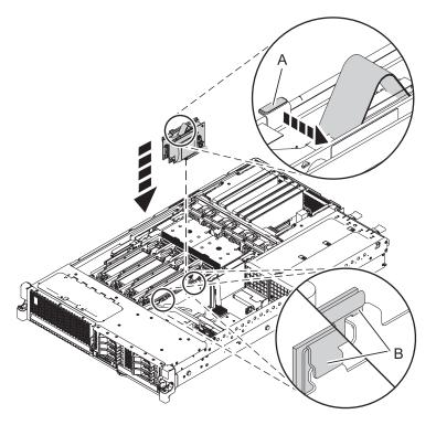
Figure 18. Replacing a RAID/cache storage controller in an 31E/1C, 31E/1D, 31E/2C, or 31E/2D
