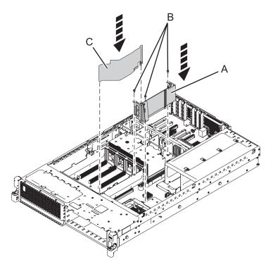
Figure 57. Replacing the voltage regulator guide air divider in the 31E/1C, 31E/1D, 31E/2C, or 31E/2D
