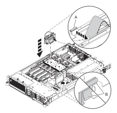
Figure 17. Replacing a RAID/cache storage controller in an 31E/2B
