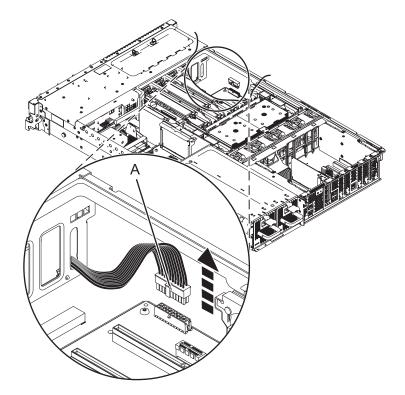
Figure 45. Removing the front fan cable
