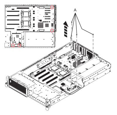
Figure 47. Removing the system backplane (four screws for 31E/1C, 31E/1D, 31E/2C, or 31E/2D)
