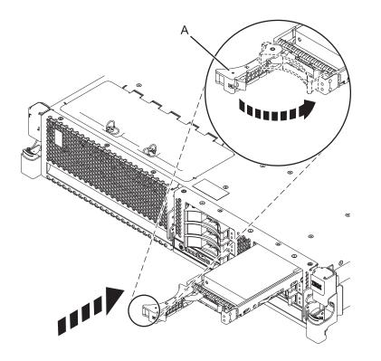
Figure 35. Installing the backplane disk drives
