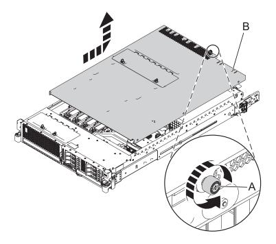
Figure 66. Removing the service access cover
