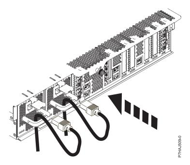
Figure 72. Connecting the power cords
