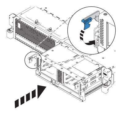
Figure 58. Replacing the disk drive cage
