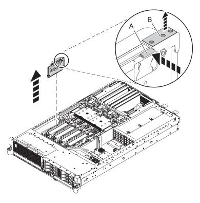
Figure 21. Removing the cache battery card for the 31E/1C, 31E/1D, 31E/2C, or 31E/2D
