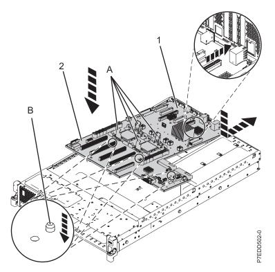
Figure 51. Replacing the system backplane in the 31E/1C, 31E/1D, 31E/2C, or 31E/2D
