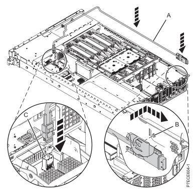
Figure 10. Installing the SAS I/O cable
