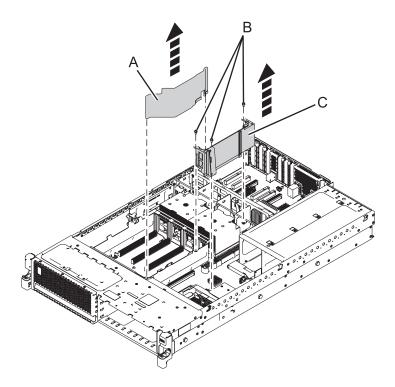
Figure 43. Removing the voltage regulator guide and air divider from the 31E/1C, 31E/1D, 31E/2C, or 31E/2D
