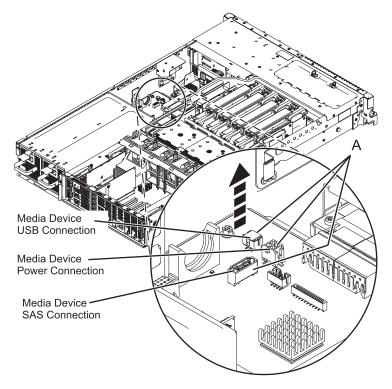
Figure 40. Disconnecting the media device cables
