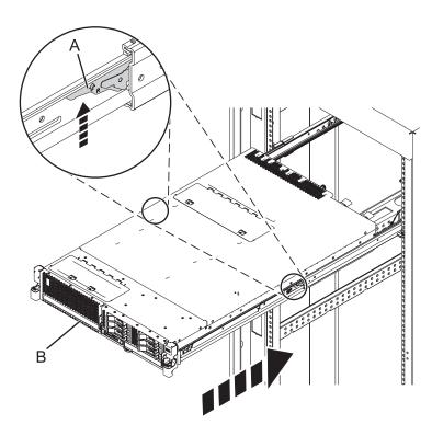
Figure 69. Unlocking the safety rail latches
