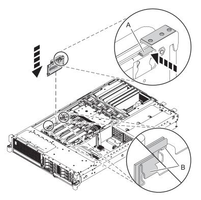
Figure 23. Installing the cache battery card for the 31E/1C, 31E/1D, 31E/2C, or 31E/2D
