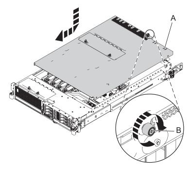
Figure 67. Installing the service access cover
