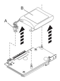
Figure 24. Removing the cache battery
