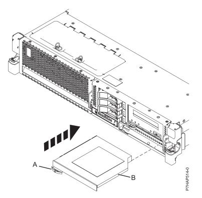
Figure 36. Installing the SAS media device
