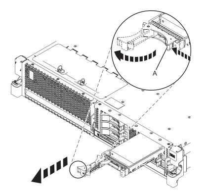
Figure 28. Removing the disk drive from the backplane
