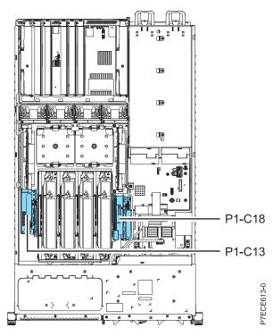
Figure 2. Slot location for storage controller and cache battery card installation for 31E/1C, 31E/1D, 31E/2C, or 31E/2D
