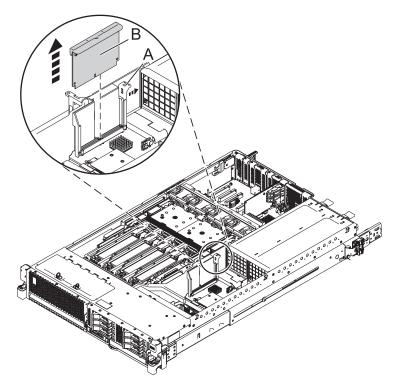
Figure 11. RAID/cache enablement card removal from a rack-mounted system unit
