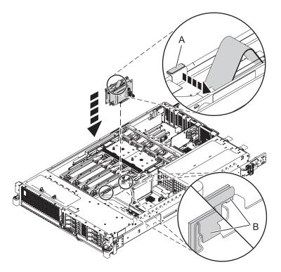
Figure 4. Replacing a RAID/cache storage controller in a rack-mounted 31E/2B
