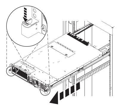
Figure 68. Placing the system in the service position
