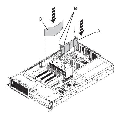
Figure 56. Replacing the voltage regulator guide air divider in the 31E/2B
