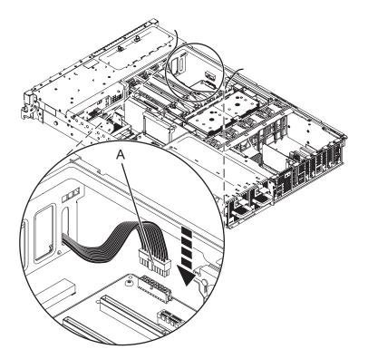
Figure 54. Connecting the fan cable
