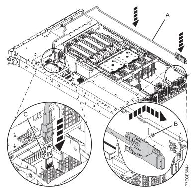
Figure 60. Replacing the SAS cable
