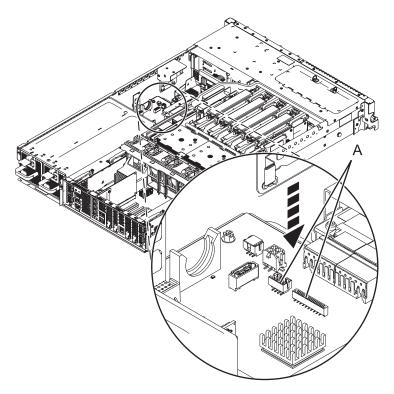
Figure 61. Connecting the operator panel cable
