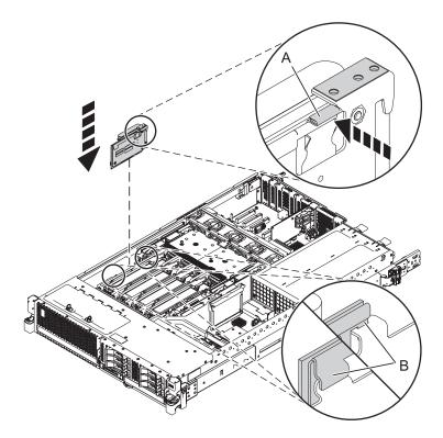
Figure 6. Cache battery card replacement for 31E/2B
