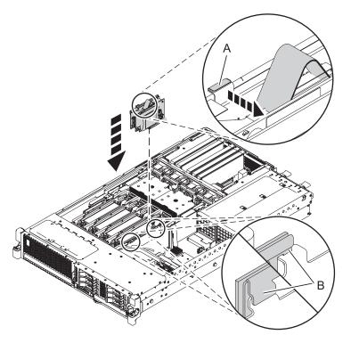
Figure 5. Replacing a RAID/cache storage controller in a rack-mounted 31E/1C, 31E/1D, 31E/2C, or 31E/2D
