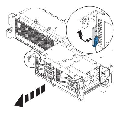
Figure 41. Removing the disk drive cage
