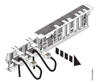
Figure 71. Removing the power cords
