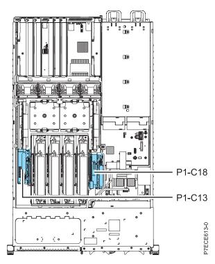
Figure 14. Slot location for storage controller (P1-C18) and cache battery card (P1-C13) installation for the 31E/1C, 31E/1D, 31E/2C, or 31E/2D
