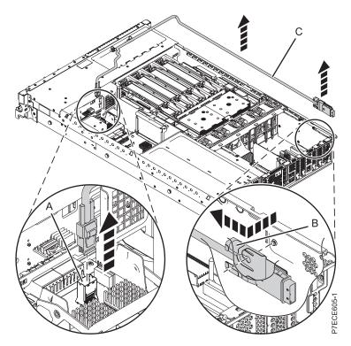
Figure 39. Removing the external SAS port
