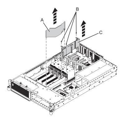
Figure 42. Removing the voltage regulator guide and air divider from the 31E/2B
