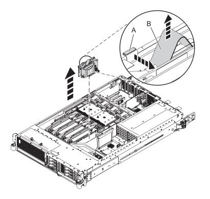
Figure 15. Removing a RAID/cache storage controller from a rack-mounted 31E/2B
