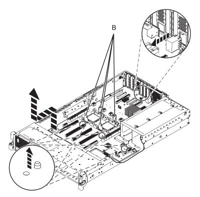
Figure 49. Removing the system backplane from the 31E/1C, 31E/1D, 31E/2C, or 31E/2D
