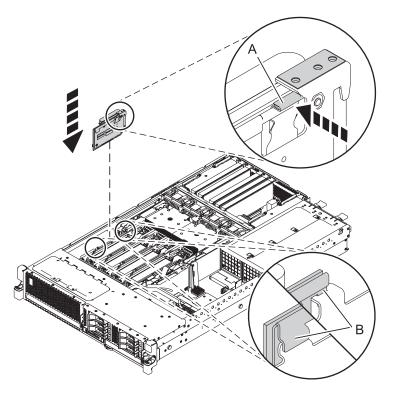
Figure 7. Cache battery card replacement for 31E/1C, 31E/1D, 31E/2C, or 31E/2D
