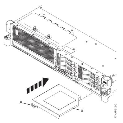
Figure 37. Installing the Slimline media device
