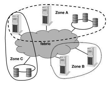
Zoning can be used as a security service, preventing some resource to be used by non authorized users: a disk subsystem with confidential data can be isolated in a zone of authorized servers. Zoning can also be used to solve some interoperability problems: a zone can be defined for all the servers and storage resources used by AIX servers, another zone being dedicated to NT servers and NT storage resources.
