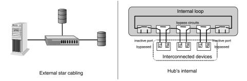
In practice, a hub may contain one or more logical loops. The repartition of ports in several loops is performed either with hardware switches, that control loop continuity or loopback, or through software configuration.
