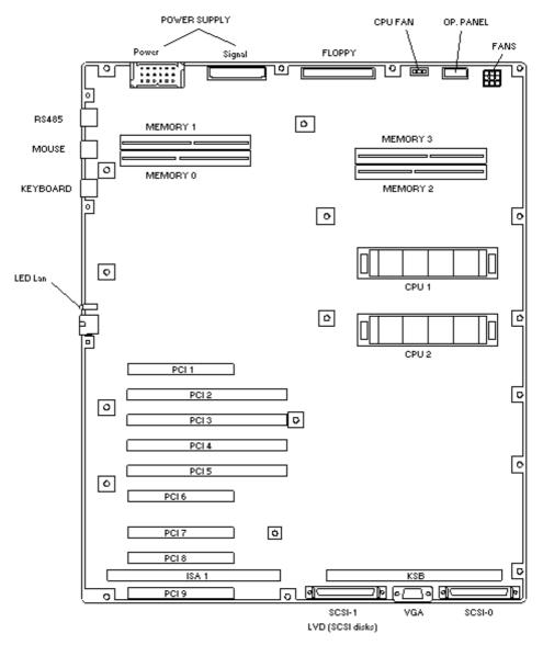
Note: The E250 planar board does not have the VGA connector.
