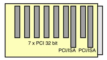
The Escala E Series Extender Card adds an additional 7 x 32-bit PCI slots and an extra 2 x PCI/ISA slots to the existing single 64-bit PCI slot included on the Planar Board. Please note however, that the 2 x PCI/ISA slots are physically overlapped with the last 2 PCI slots. This means that a maximum of 7 slots may be occupied at any one time, i.e. the 2 x PCI/ISA and 2 x PCI are mutually exclusive.
