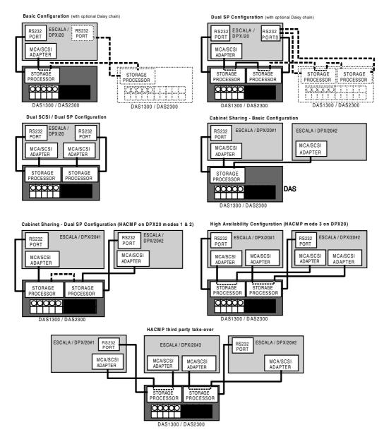
Performance in these configurations is dictated by a number of factors, including host CPU utilization, SCSI bus traffic, individual disk usage, write cache option.
