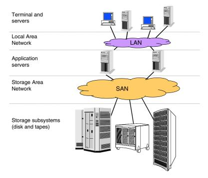
In the literature, the term SAN refers either to the high speed network infrastructure, or may cover the whole storage architecture, including servers, storage subsystems and management software.
