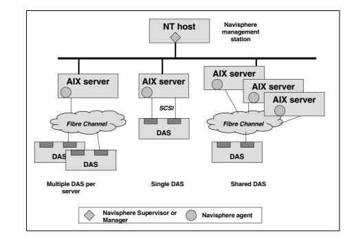
The next figure shows a sample of Navisphere Supervisor or Manager deployment, to manage DAS subsystems connected to AIX servers.
