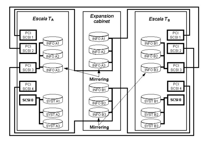
The base of the native HA feature is the RAID 1 software provided by the AIX® mirroring, along with the double master Ultra Wide SCSI bus. In normal operations, both systems are running their own part of the application workload. If one of the two systems fails despite all internal RAS protections, thanks to HA-CMP software, the second system running the other part of the application is able to take over the workload of the first system.
