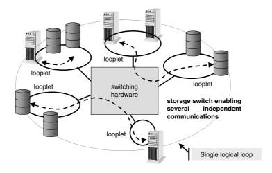
This kind of features can be available in managed hubs relying on an internal switching architecture, or can be emulated on fabric switches. Depending on the implementations, the logical loop can be limited to a single hub/switch, or can spawn across multiple hubs/switches.
