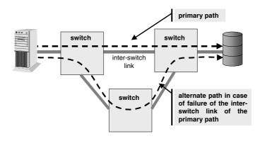
Multiple inter-switch links can be aggregated, to avoid the risk of bandwidth bottleneck that may arise when using a single link operating at the same speed than the switch ports.
