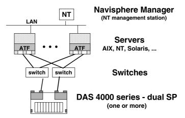
There is a version of Access Logix for each DAS product (4500, 4700 and 4700-2). Access Logix provides the same features on all subsystems.
