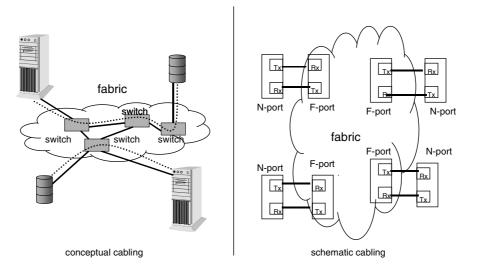
Integrated routing algorithms automatically route circuits and frames across the fabric, through the best path. Resilient multi-switch fabrics can be deployed, with automatic data routing and re-routing, self-healing and almost unlimited scalability.
