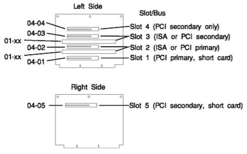
Note: The xx digits in the ISA slot location codes are determined by the order in which the ISA adapters are configured.
