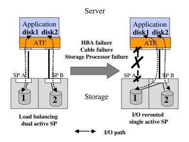
In the unlikely event of a failure, the failover occurs in seconds, permitting continuous access to the information stored on the disk subsystem(s). Without the user intervention, ATF reconfigures the RAID subsystem (e.g. bind the LUNs to the surviving SP), retrieves I/Os in the mirrored write cache and completes them, and finally, on the server it self, route the I/O through a secondary path to the surviving (provided that the server is equipped with two fibre channel adapters).
