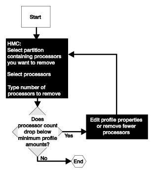
To remove processor resources from an active partition without rebooting the partition, do the following:
