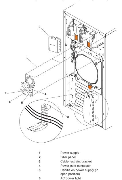
**Note:** You do not need to turn off the power to the system to install hot-swap power supplies if your system has a redundant (third) power supply installed.
