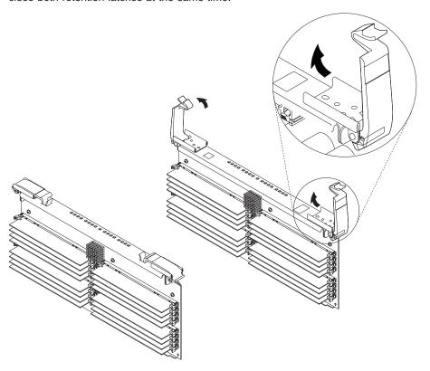
2. Align the card with the card guides and card connector.
