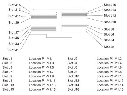
3. Remove the memory DIMM by pushing the tabs out on the memory connectors.
