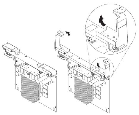
2. Align the card with the card guides and card connector.
