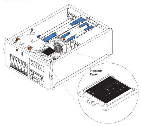
The following illustration shows the LEDs on the indicator panel, located inside the server.
