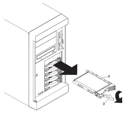
2. Remove the disk drive (1) by placing the handle (2) on the drive to the open position (perpendicular to the drive) and pulling the hot-swap tray from the bay.
