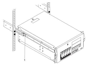
After completing actions, return the system to the normal position by pressing in on the safety latches (1).
