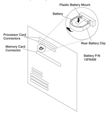
9. Pry the battery out of its mount using your fingernail. After the top of the battery has cleared the plastic mount, pull it up and out of the system board.
