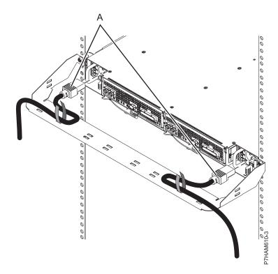
Figure 6. Installing the power cords
