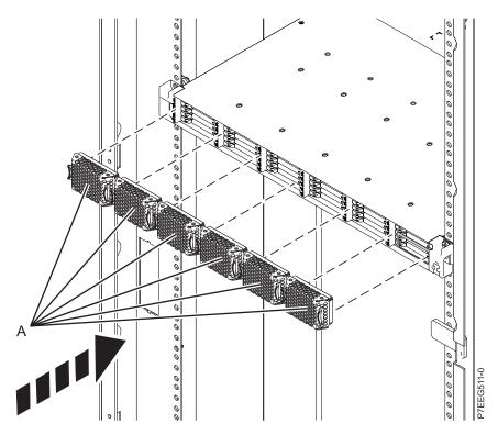
Figure 5. Installing the SSD EMC bezels
