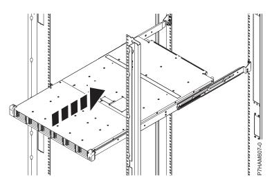
Figure 15. Sliding the disk drive enclosure into the rack
