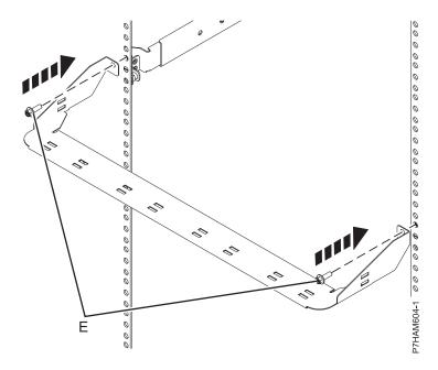
Figure 12. Mounting the cable management bracket
