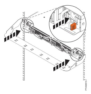
Figure 3. Docking the power supply
