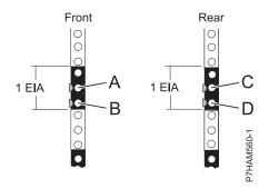
Figure 8. Marking the installation locations
