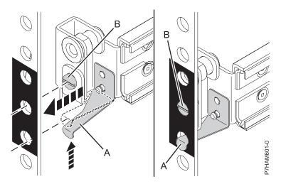
Figure 9. Mounting the rail to the front of the rack
