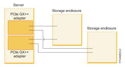
Figure 23. Example of a server that has two PCIe GX++ adapters connected to two storage enclosures for high availability
