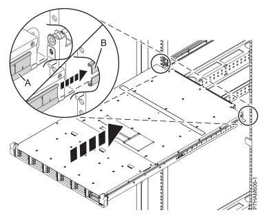
Figure 14. Fitting the enclosure into the rail sheath
