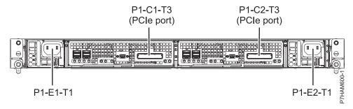
Figure 30. Model 58/88 connector locations
