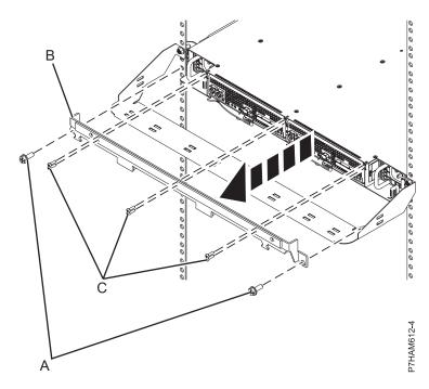
Figure 2. Removing the rear shipping bracket
