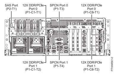
Figure 26. Model 05E/6C connections for expansion units, disk drive enclosures, and PCIe storage enclosures
