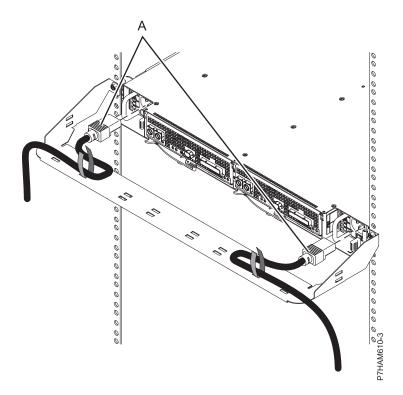
Figure 19. Installing the power cords
