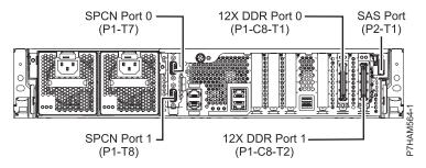
Figure 28. Model 31E/2C connections for expansion units and disk drive enclosures
