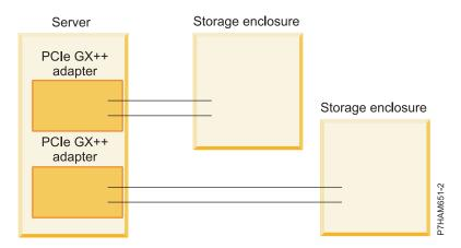
Figure 21. Example of a server that has two PCIe GX++ adapters connected to two storage enclosures
