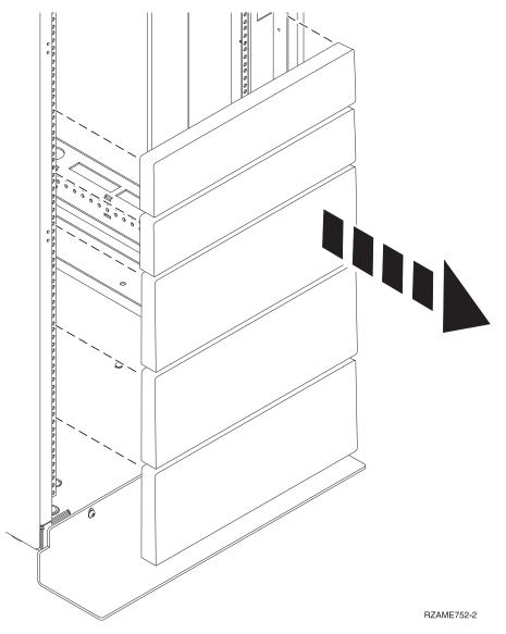
Figure 7. Removing the filler panels
