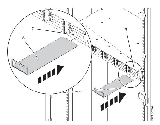
Figure 17. Inserting the service card
