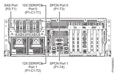
Figure 25. Model 02E/4C connections for expansion units, disk drive enclosures, and PCIe storage enclosures
