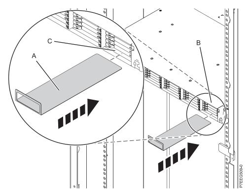
Figure 4. Inserting the service card
