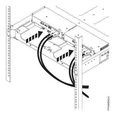
Figure 3. Sliding the ESM units toward the chassis
