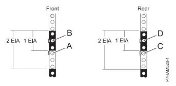
Figure 16. Marking the installation locations
