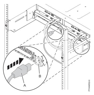
Figure 13. Connecting the power supply line cords
