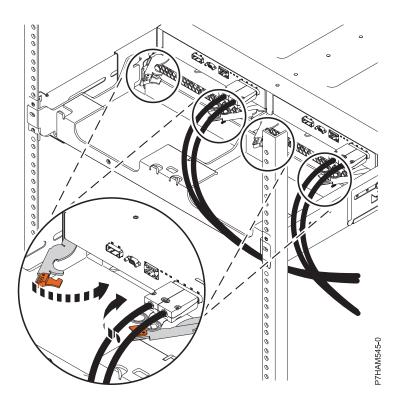
Figure 6. Closing the ESM release levers
