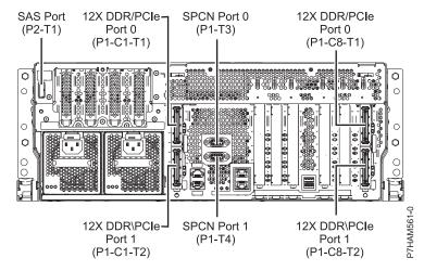
Figure 45. Model 05E/6C connections for expansion units, disk drive enclosures, and PCIe storage enclosures
