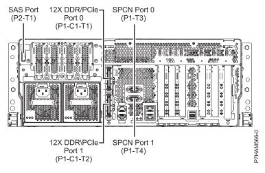
Figure 41. Model 02E/4C connections for expansion units, disk drive enclosures, and PCIe storage enclosures
