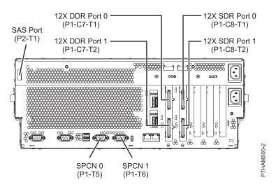
Figure 54. Model 33E/8B connector locations on a rack-mounted model
