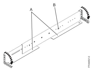
Figure 18. Opening the rail hinge bracket
