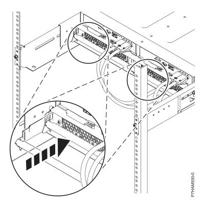
Figure 11. Docking the power supplies
