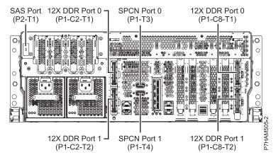
Figure 43. Model 05F/6B connector locations on a rack-mounted model
