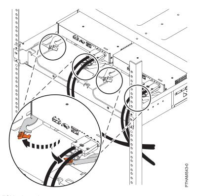
Figure 4. Opening the ESM release levers
