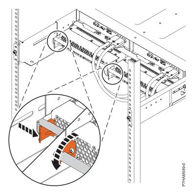
Figure 10. Opening the power supply release handle
