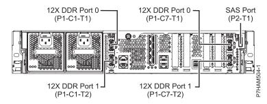
Figure 49. Model 31E/2B connector locations on a rack-mounted model
