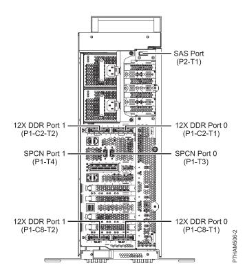
Figure 44. Model 05F/6B connector locations on a stand-alone model
