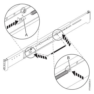
Figure 17. Installing the spring to the rail
