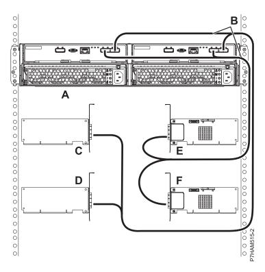
Figure 37. Mode 4 connection of one 58/87 disk drive enclosure by using X cables to four independent SAS adapters
