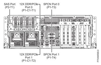
Figure 42. Model 02E/4D connections for expansion units, disk drive enclosures, and PCIe storage enclosures
