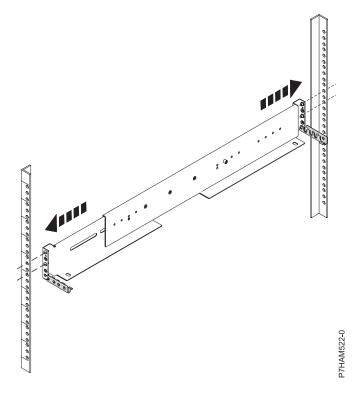
Figure 19. Mounting the rail on the rack
