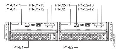
Figure 61. Model 58/87 connector locations
