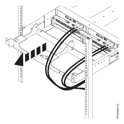
Figure 8. Removing the large bracket
