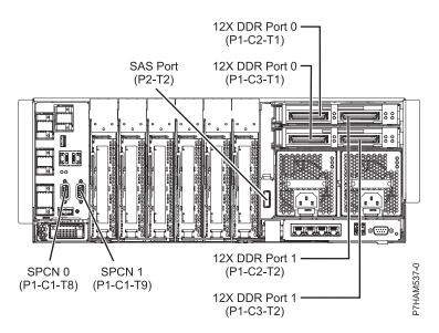
Figure 60. Model 17M/MD or 79M/HD connector locations
