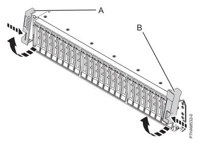
Figure 21. Removing the side bezels
