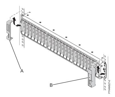
Figure 25. Attaching the side bezels
