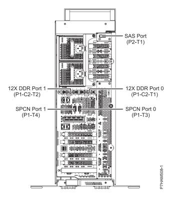
Figure 40. Model 02E/4B connector locations on a stand-alone model
