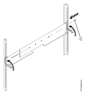
Figure 20. Securing the rail to the rack
