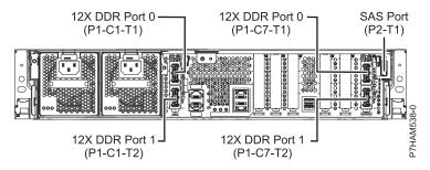
Figure 55. Model 46L/1S connector locations
