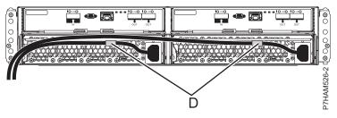
Figure 14. Routing the power cords through the cord retention brackets
