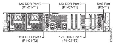
Figure 56. Model 46L/2S connector locations
