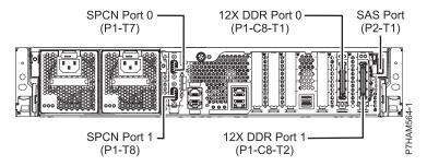
Figure 52. Model 31E/2D connections for expansion units and disk drive enclosures
