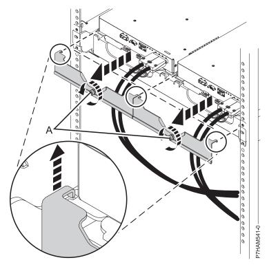
Figure 2. Removing the small front brackets
