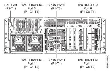
Figure 46. Model 05E/6D connections for expansion units, disk drive enclosures, and PCIe storage enclosures
