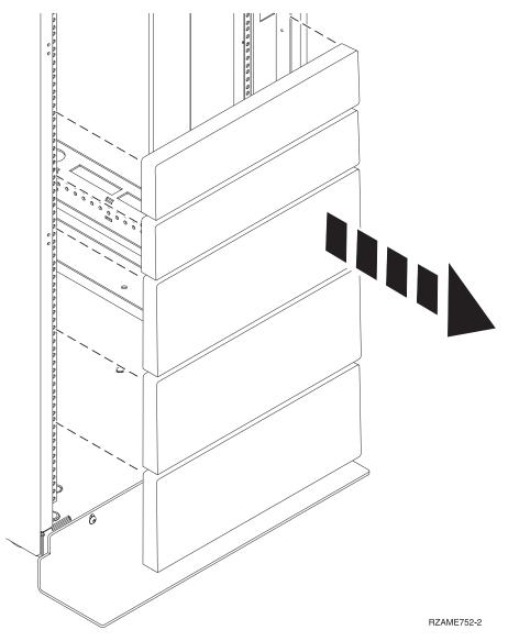
Figure 15. Removing the filler panels
