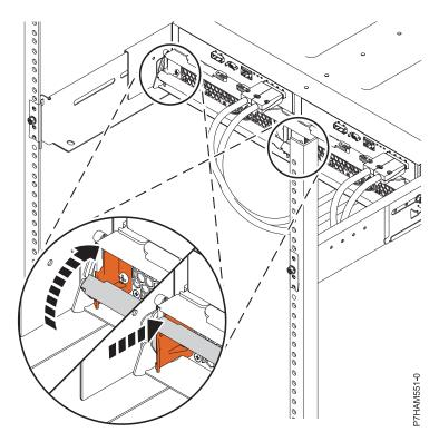
Figure 12. Closing the power supply release handle
