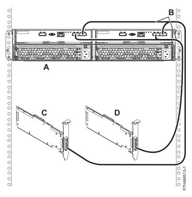
Figure 35. Mode 2 connection of one 58/87 disk drive enclosure by using YO cables to two independent SAS adapters
