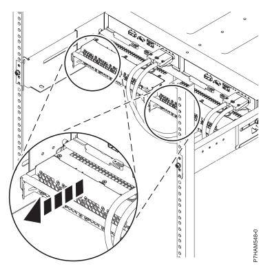
Figure 9. Sliding the power supplies toward the chassis
