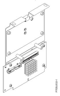
Figure 15. CCIN 2BE1 PCI-X266 Planar 3 Gb SAS RAID adapter
