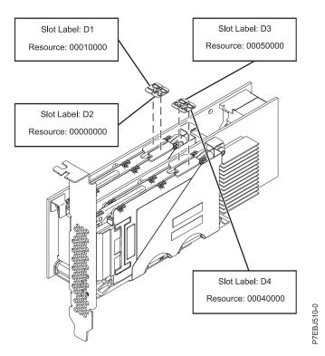
Figure 11. CCIN 57CD PCIe SAS RAID and SSD adapter 3 Gb x8
