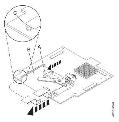
Figure 26. Removing the cache battery
