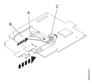
Figure 27. Replacing the cache battery
