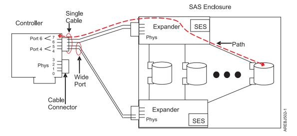
Figure 16. Example of the SAS subsystem
