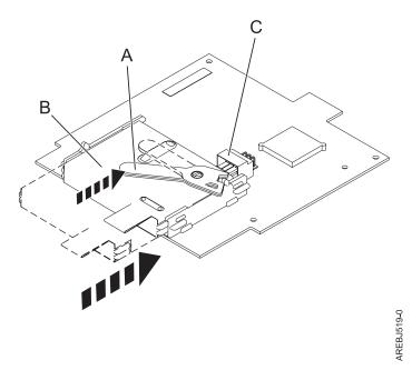
Figure 25. Replacing the cache battery
