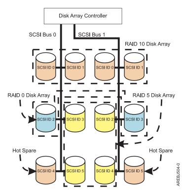
Figure 17. Disk array configuration
