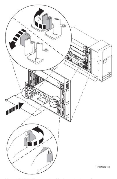
Figure 139. PCI adapter replaced in the stand-alone unit
