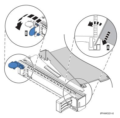
Figure 88. Placing the PCI adapter single-width cassette
