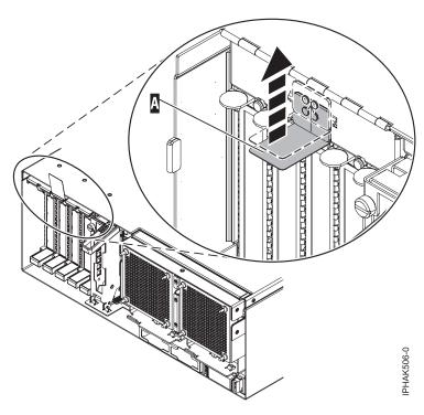
Figure 68. Lift up the EMC shield
