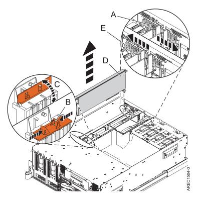
Figure 6. PCI adapter removal
