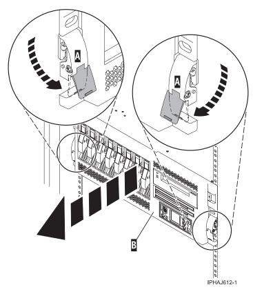
Figure 177. Releasing the rack latches
