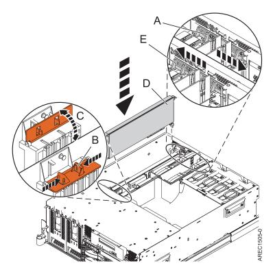
Figure 11. PCI adapter installation
