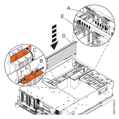
Figure 4. PCI adapter installation
