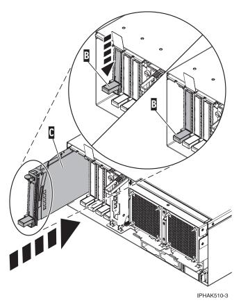
Figure 71. PCI adapter cassette removed from the system unit
