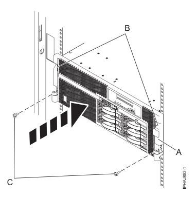
Figure 179. Pushing the system into the rack and attaching the thumbscrews
