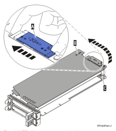
Figure 119. PCI adapter cassette cover replaced
