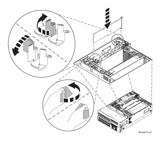
Figure 156. PCI adapter replaced in the rack-mounted system unit
