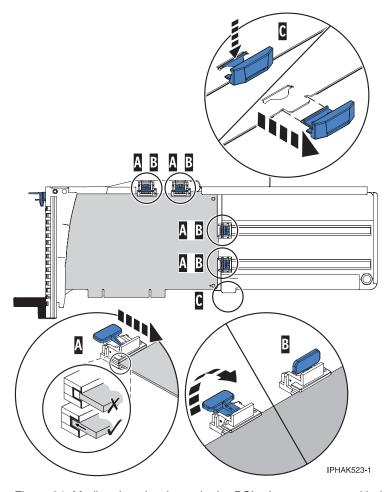
Figure 84. Medium-length adapter in the PCI adapter cassette with the supports in place
