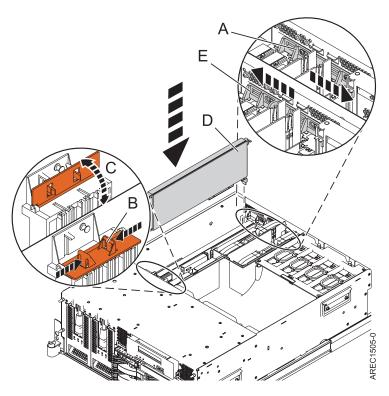
Figure 9. PCI adapter installation
