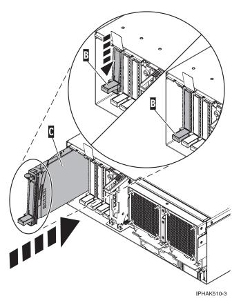
Figure 66. PCI adapter cassette removed from the system unit
