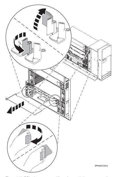
Figure 143. PCI adapter removed from the stand-alone system unit
