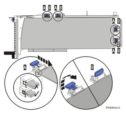
Figure 122. Long adapter in the PCI adapter cassette with the supports and stabilizer in place
