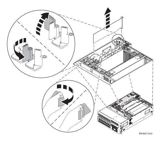
Figure 140. PCI adapter removed from the rack-mounted system unit
