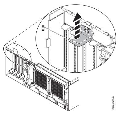
Figure 57. Lift up the EMC shield
