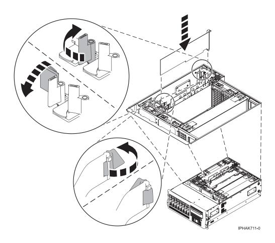
Figure 138. PCI adapter replaced in the rack-mounted unit
