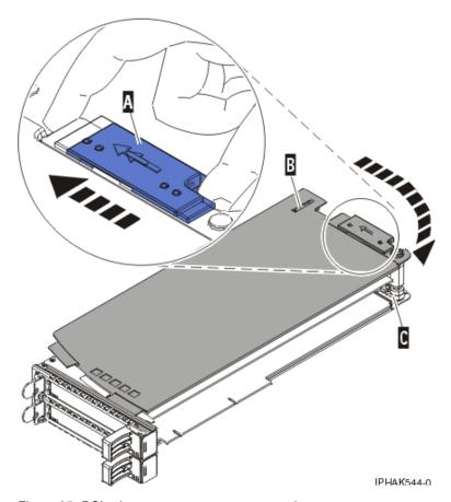
Figure 95. PCI adapter cassette cover removed
