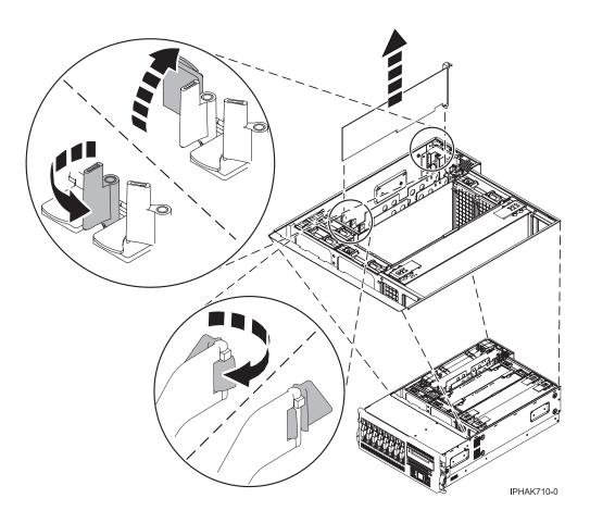
Figure 124. PCI adapter or filler plate removed from the rack-mounted unit
