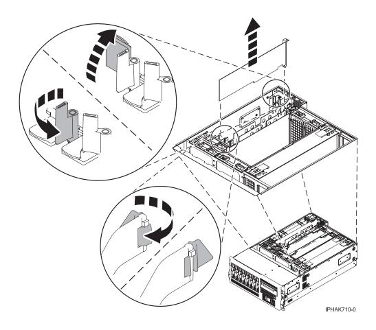
Figure 136. PCI adapter or filler plate removed from the rack-mounted unit
