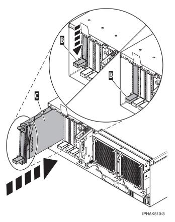
Figure 43. PCI adapter cassette removed from the system unit
