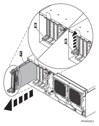
Figure 59. PCI adapter cassette removed from the system unit
