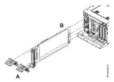
Figure 91. Replace the cassette and install the EMC grill
