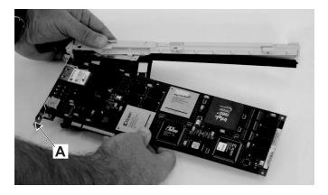
Remove the adapter from the cassette linkage assembly by rotating the bottom of the tailstock A out as shown in the illustration. Store the adapter in a safe place.
