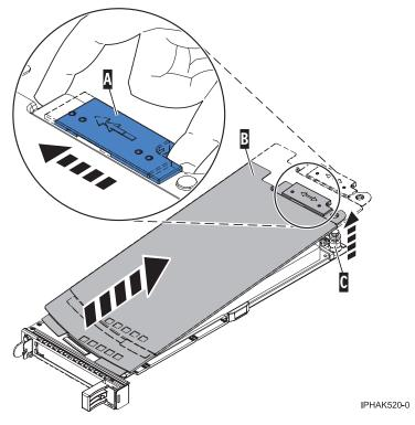
Figure 92. PCI adapter cassette cover removed
