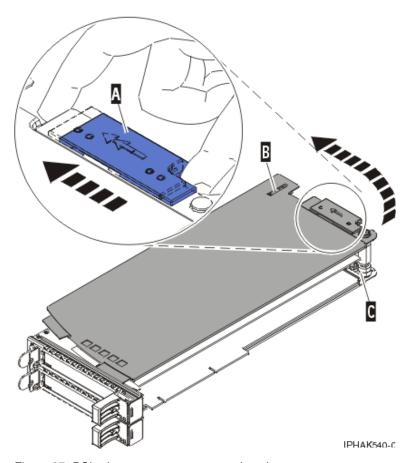
Figure 97. PCI adapter cassette cover replaced
