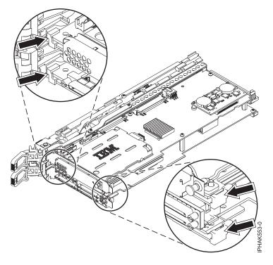
b. Attach the rear arms of the cassette assembly to the notches at the rear end of the double-wide adapter.
