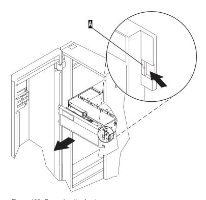
Figure 165. Removing the front cover
