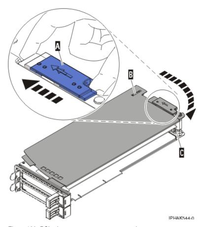
Figure 120. PCI adapter cassette cover removed
