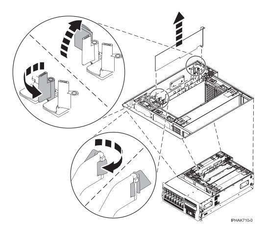
Figure 128. PCI adapter or filler plate removed from the rack-mounted unit
