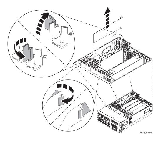
Figure 144. PCI adapter removed from the rack-mounted unit
