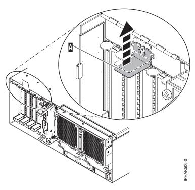
Figure 45. Lift up the EMC shield
