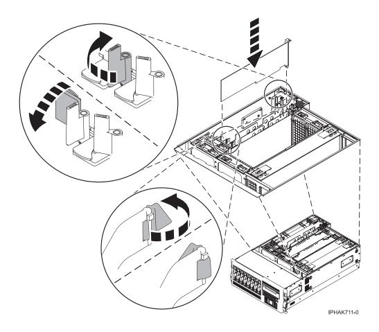
Figure 130. PCI adapter replaced in the rack-mounted unit
