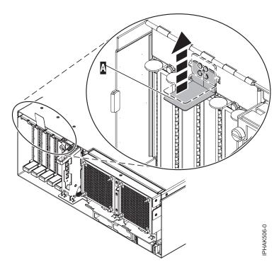
Figure 40. Lift up the EMC shield
