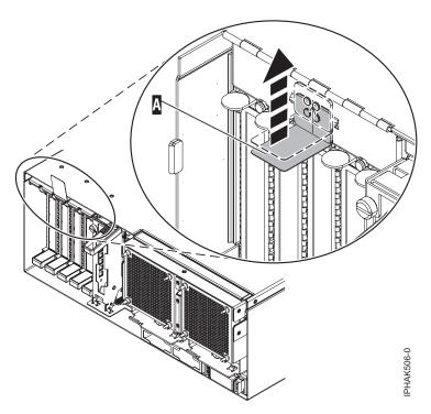
Figure 73. Lift up the EMC shield
