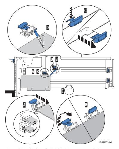
Figure 85. Small adapter in the PCI adapter cassette with the supports and the hookarm in place
