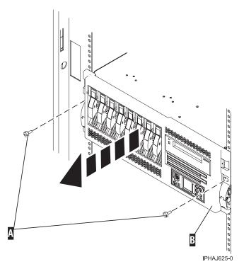
Figure 176. Removing the thumbscrews from the system and rack
