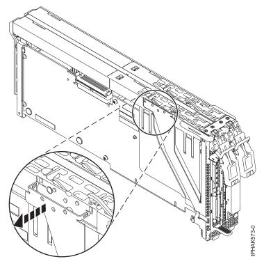
7. Detach the tab at the bottom of the cassette assembly from the notches on the face plate and lift up on the locking arms.
