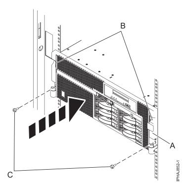
Figure 171. Installing the front cover on a rack-mounted model
