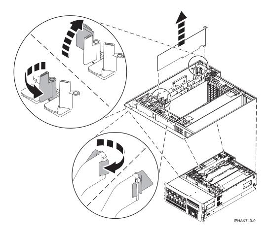
Figure 132. PCI adapter or filler plate removed from the rack-mounted unit
