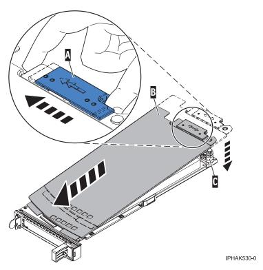
Figure 86. PCI adapter cassette cover replaced
