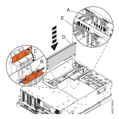
Figure 12. PCI adapter installation
