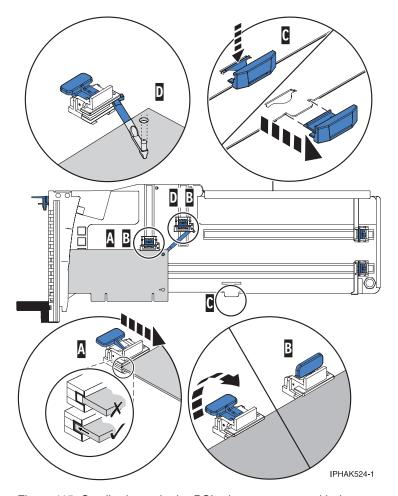
Figure 115. Small adapter in the PCI adapter cassette with the supports and the hookarm in place
