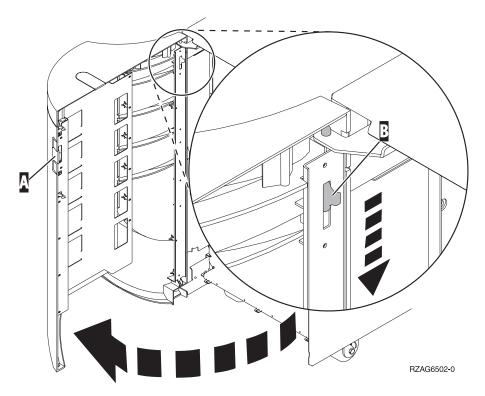
Figure 160. Removing the expansion unit rear door
