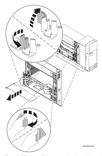
Figure 133. PCI adapter or filler plate removed from the stand-alone unit
