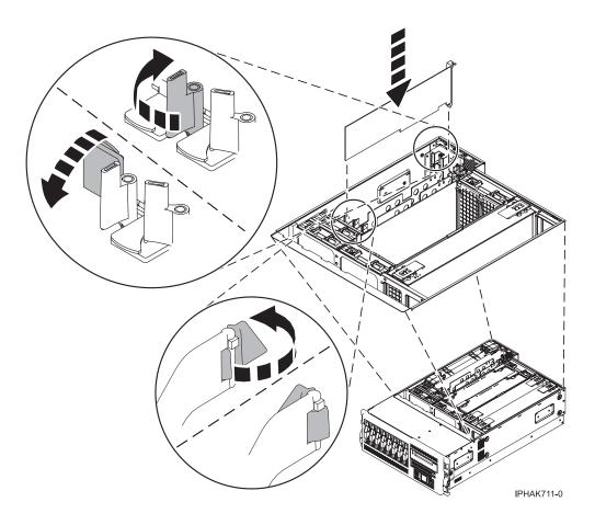
Figure 148. PCI adapter replaced in the rack-mounted unit
