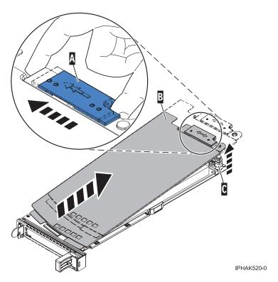
Figure 106. PCI adapter cassette cover removed
