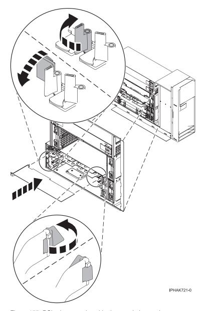
Figure 155. PCI adapter replaced in the stand-alone unit
