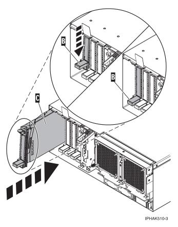
Figure 48. PCI adapter cassette removed from the system unit
