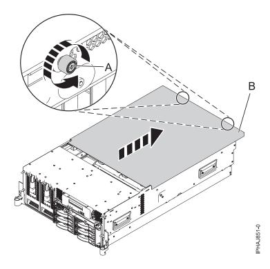
Figure 166. Remove the service access cover from a rack-mounted model
