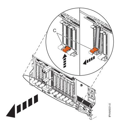
Figure 105. Removing a PCI adapter cassette
