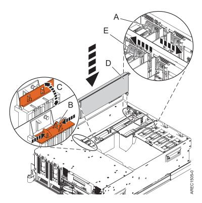
Figure 2. PCI adapter installation
