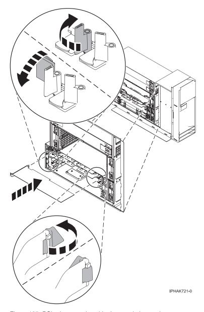
Figure 135. PCI adapter replaced in the stand-alone unit
