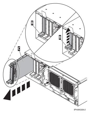
Figure 65. PCI adapter cassette removed from the system unit
