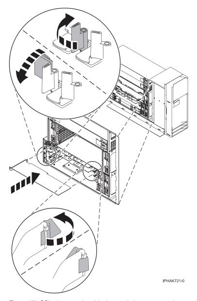
Figure 157. PCI adapter replaced in the stand-alone system unit
