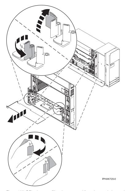
Figure 125. PCI adapter or filler plate removed from the stand-alone unit
