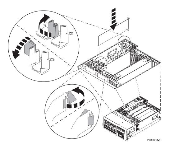
Figure 154. PCI adapter replaced in the rack-mounted unit
