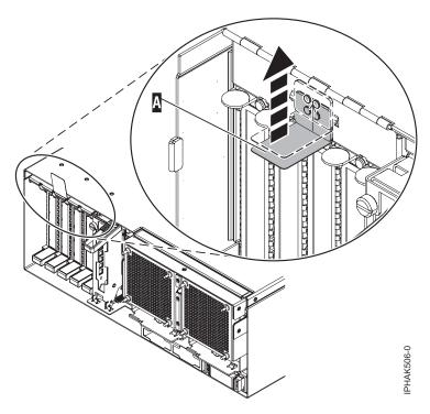
Figure 60. Lift up the EMC shield
