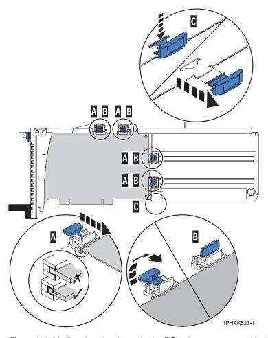
Figure 114. Medium-length adapter in the PCI adapter cassette with the supports in place
