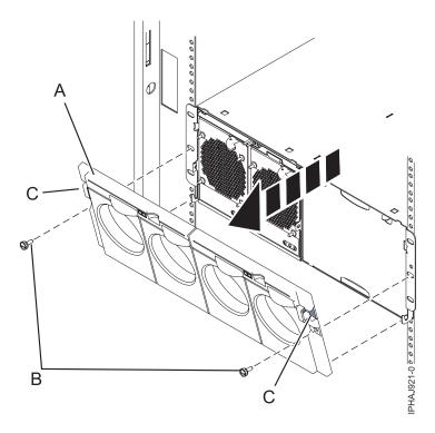
Figure 162. Remove the front cover for model 7314-G30 or 5796
