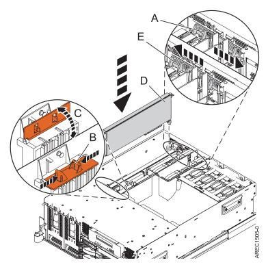
Figure 13. PCI adapter installation
