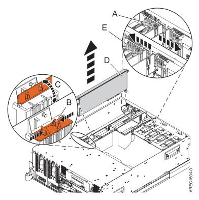
Figure 5. PCI adapter removal
