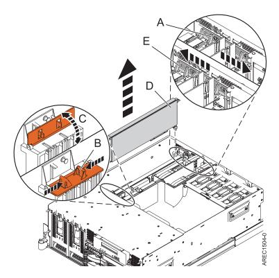
Figure 7. PCI adapter removal
