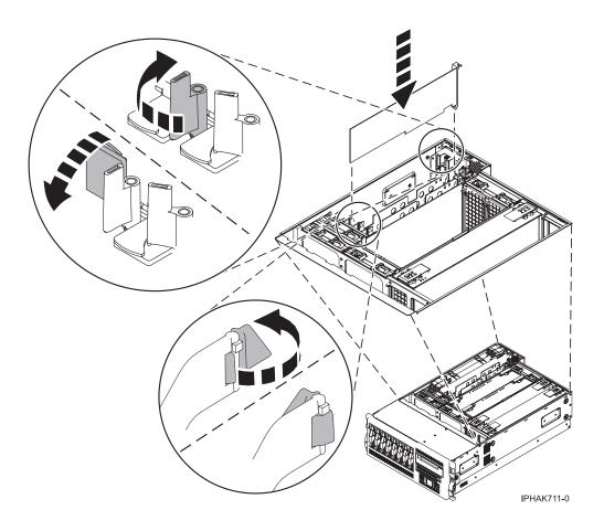
Figure 152. PCI adapter replaced in the rack-mounted system unit
