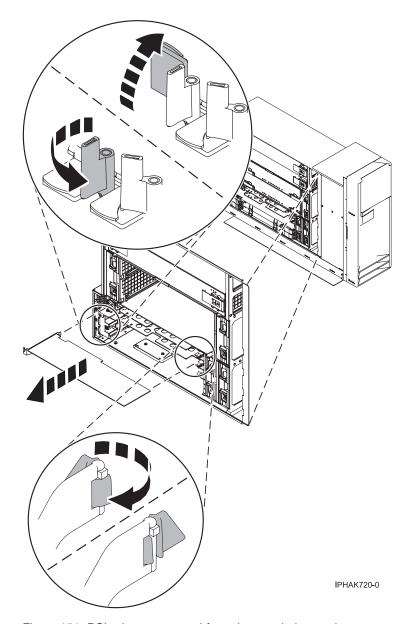
Figure 151. PCI adapter removed from the stand-alone unit
