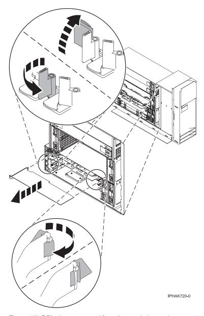
Figure 147. PCI adapter removed from the stand-alone unit
