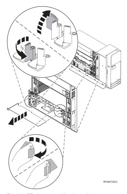
Figure 141. PCI adapter removed from the stand-alone unit
