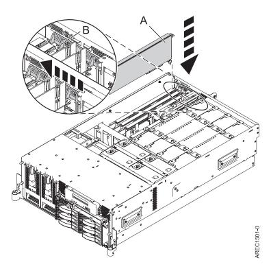
Figure 19. PCI adapter replaced in the rack-mounted system unit
