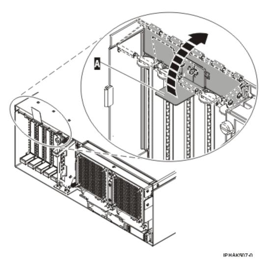
Figure 46. Rotate the EMC shield into the open position
