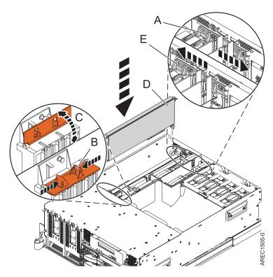
Figure 3. PCI adapter installation
