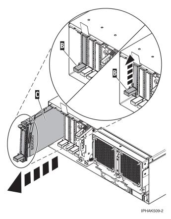
Figure 47. PCI adapter cassette removed from the system unit.
