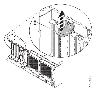
Figure 63. Lift up the EMC shield
