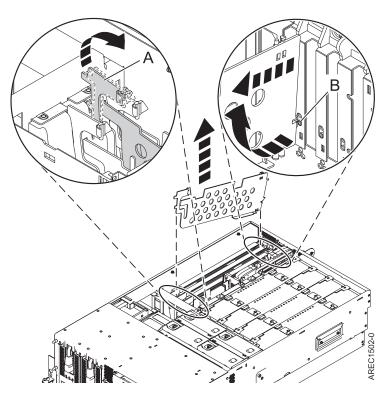
Figure 33. PCI-adapter divider removed from the system unit
