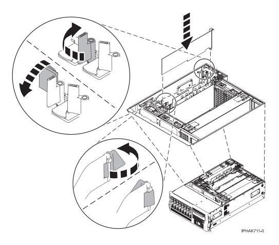
Figure 134. PCI adapter replaced in the rack-mounted unit
