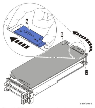
Figure 101. PCI adapter cassette cover replaced
