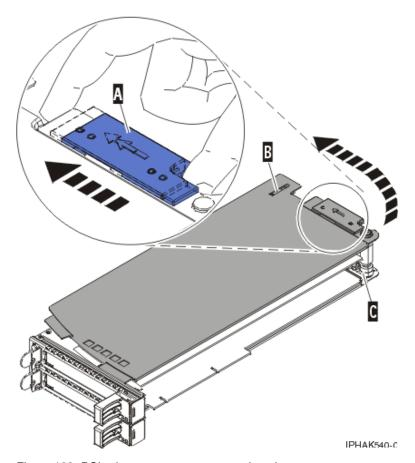
Figure 123. PCI adapter cassette cover replaced
