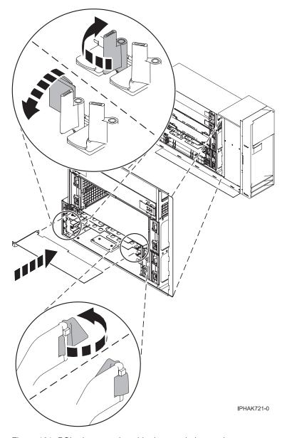
Figure 131. PCI adapter replaced in the stand-alone unit
