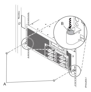
Figure 180. Releasing the rack latches
