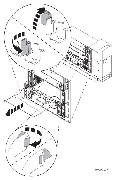
Figure 129. PCI adapter or filler plate removed from the stand-alone unit
