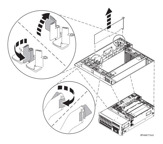
Figure 142. PCI adapter removed from the rack-mounted system unit
