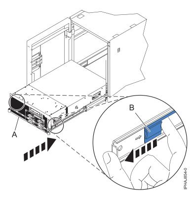
Figure 181. Releasing the rail safety latches
