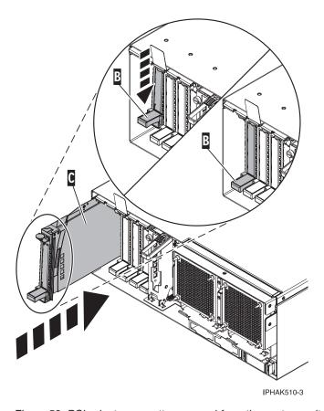
Figure 53. PCI adapter cassette removed from the system unit
