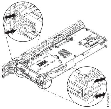
b. Detach the rear arms of the cassette assembly from the notches at the rear end of the double-wide adapter.
