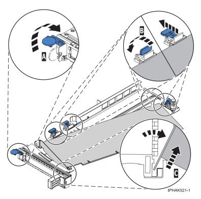
Figure 107. Adapter removed from the PCI adapter cassette
