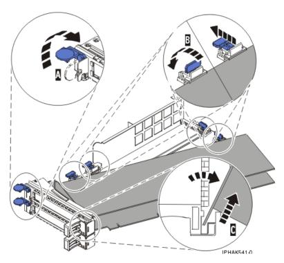
Figure 118. Adapter removed from the PCI adapter cassette
