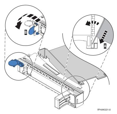
Figure 82. Adapter removed from the PCI adapter single-width cassette
