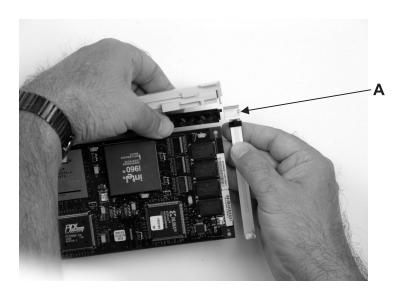
Each adapter arm has a release tab A that allows the arm to be moved away from the adapter in the cassette assembly. Use your fingernail to lift the tab, which allows the arm to be moved away from the adapter. Lift the release tab on the large adapter arm, and slide it off the cassette linkage assembly.
