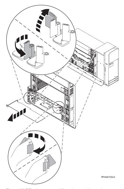
Figure 145. PCI adapter removed from the stand-alone unit
