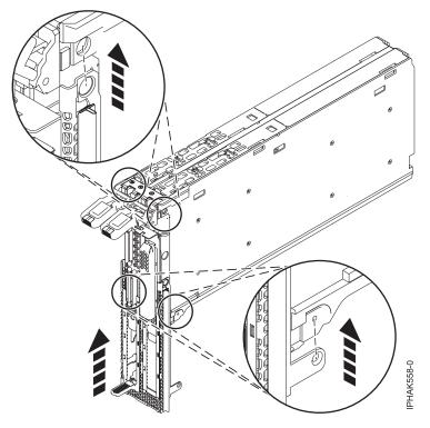
7. Press the locking arms down and insert the tab at the bottom of the cassette assembly into the notches on the face plate.
