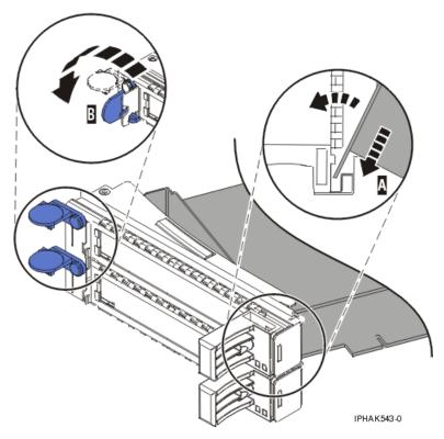
Figure 121. Adapter replaced in the PCI adapter cassette
