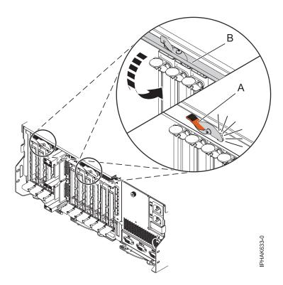
Figure 103. Closing the access door
