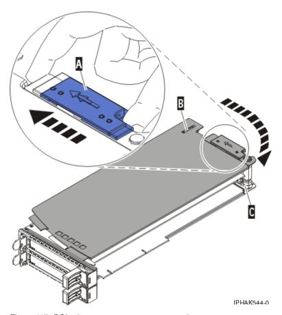
Figure 117. PCI adapter cassette cover removed
