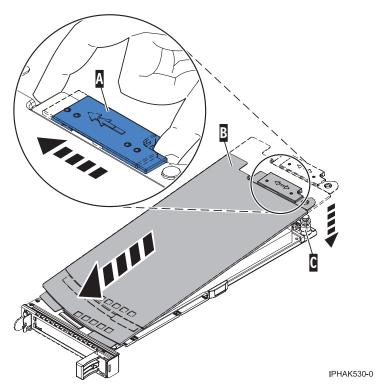
Figure 116. PCI adapter cassette cover replaced
