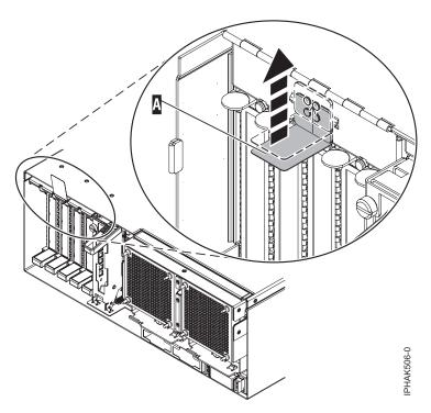
Figure 50. Lift up the EMC shield
