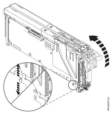
8. Remove the face plate from the front of the cassette assembly. Ensure that the top of the face plate detaches from the notches on both the front and sides of the cassette assembly.
