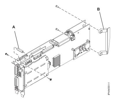
2. Align the double-wide adapter with the cassette assembly so that the spacer on the cassette assembly fits between the two sides of the double-wide adapter.
