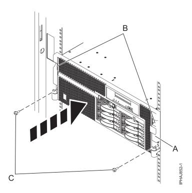
Figure 182. Replacing the thumbscrews
