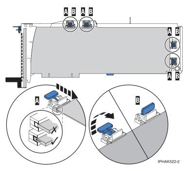
Figure 113. Large adapter in the PCI adapter cassette with the supports and stabilizer in place
