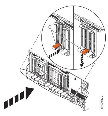
Figure 102. Installing the PCI adapter cassette
