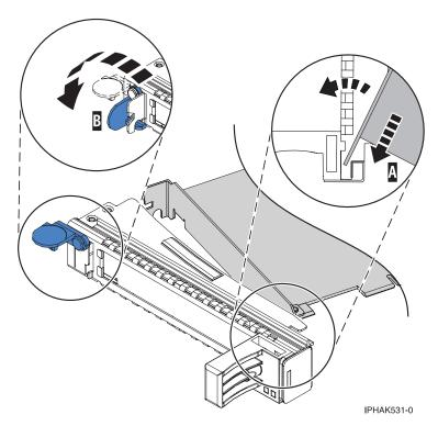
Figure 112. Adapter removed from the PCI adapter single-width cassette
