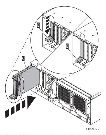
Figure 75. PCI adapter cassette removed from the system unit
