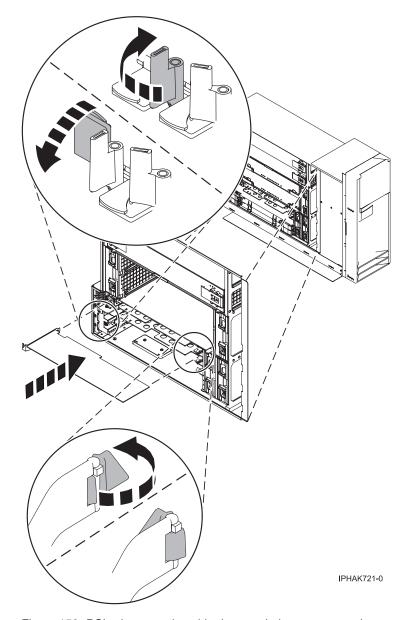
Figure 153. PCI adapter replaced in the stand-alone system unit
