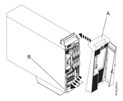
Figure 173. Replacing the cover on the model
