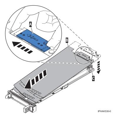
Figure 94. PCI adapter cassette cover replaced
