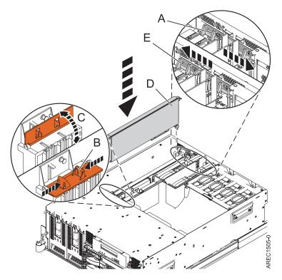
Figure 1. PCI adapter installation
