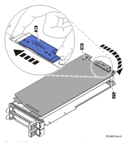
Figure 98. PCI adapter cassette cover removed
