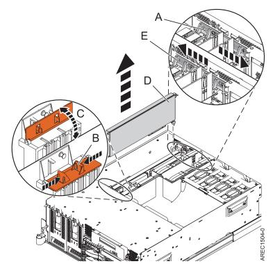
Figure 10. PCI adapter removal
