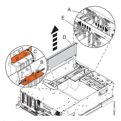
Figure 8. PCI adapter removal
