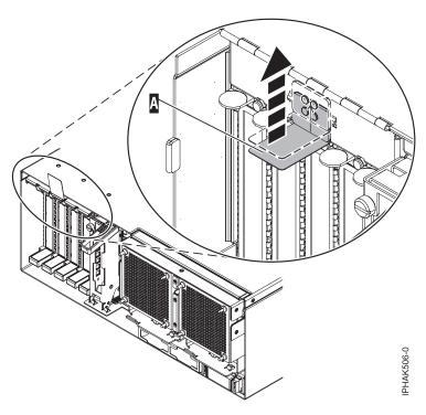
Figure 35. Lift up the EMC shield
