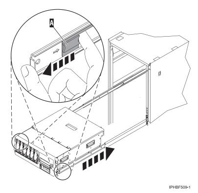
Figure 178. Releasing the rail safety latches
