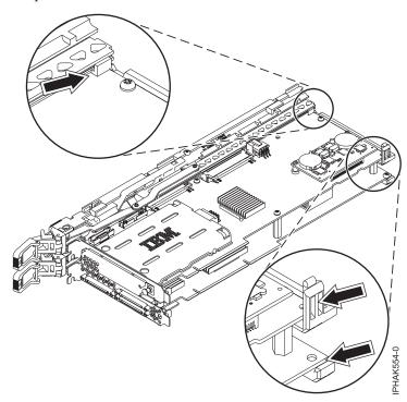
4. Secure the lower, rear arm of the cassette assembly to the rear end of the double-wide adapter using the small screw.
