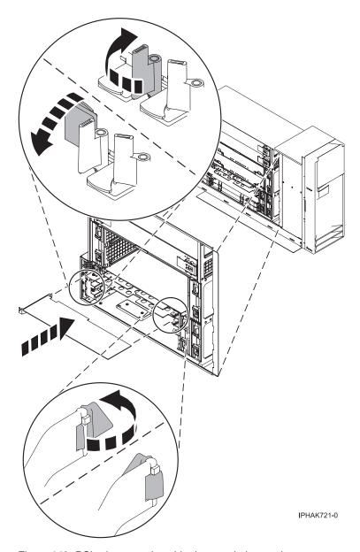
Figure 149. PCI adapter replaced in the stand-alone unit
