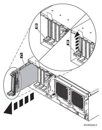
Figure 56. PCI adapter cassette removed from the system unit
