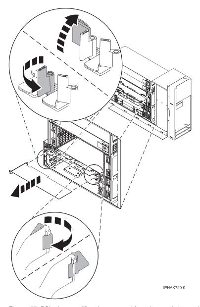
Figure 137. PCI adapter or filler plate removed from the stand-alone unit
