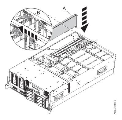
Figure 31. PCI adapter replaced in the rack-mounted system unit
