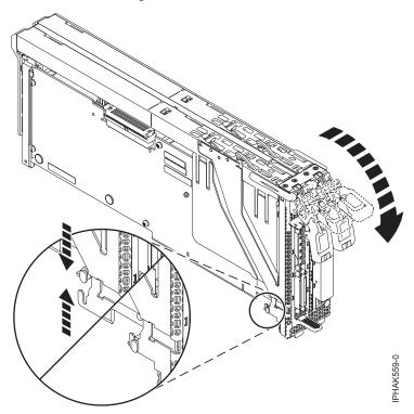
8. Press the outer arms of the face plate assembly into place.
