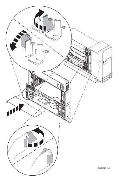
Figure 127. PCI adapter replaced in the stand-alone unit
