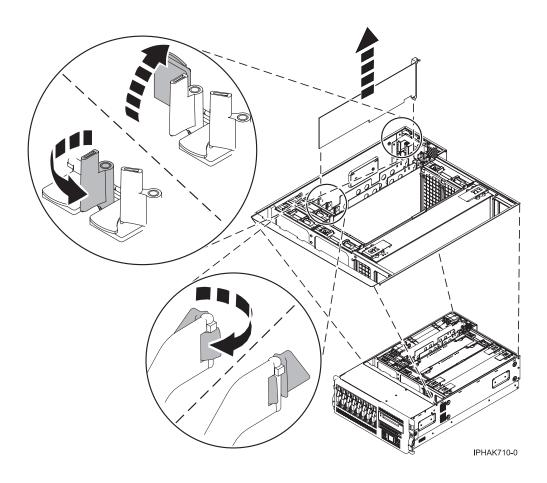
Figure 146. PCI adapter removed from the rack-mounted unit
