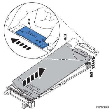
Figure 79. PCI adapter single-width cassette cover removed
