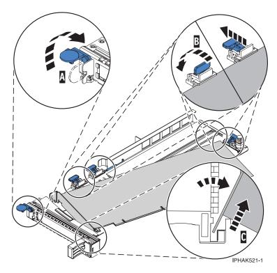
Figure 93. Adapter removed from the PCI adapter cassette
