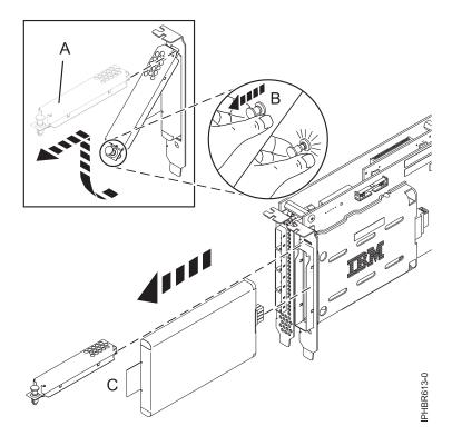
Figure 28. Replacing the 572F/575C cache battery
