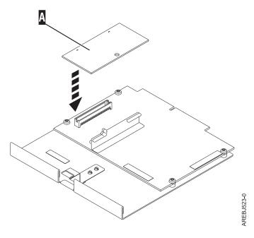
5. Install the controller using the installation procedures for the model or expansion unit on which you are working.
