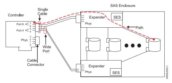
Figure 16. Example SAS subsystem
