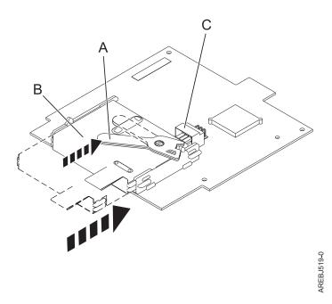
Figure 26. Replacing the 57B7 cache battery
