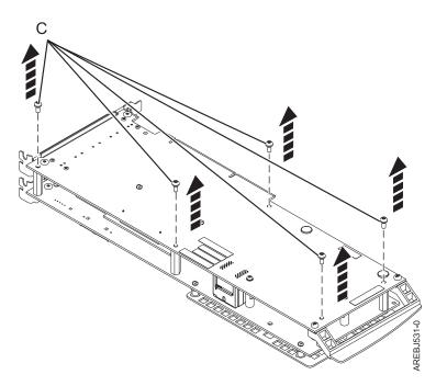
Figure 30. Location of screws on the 572F/575C card set adapter
