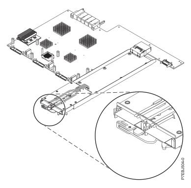
Figure 15. CCIN 57CF PCI Express x8 Planar 3 Gb SAS RAID Adapter
