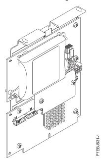
Figure 7. CCIN 2BE1 PCI-X266 Planar 3 Gb SAS RAID Adapter
