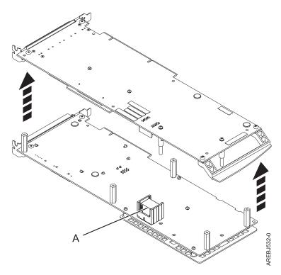
Figure 31. Location of interconnect connector on the 572F/575C card set adapter
