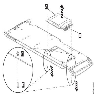
Figure 24. Removing the cache battery
