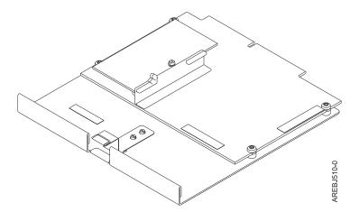
Figure 4. CCIN 57B8 planar RAID enablement card
