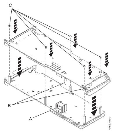
Figure 34. Reassembling the cards
