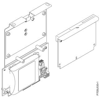
Figure 5. CCIN 2BE0 PCI-X266 Planar 3 Gb SAS Adapter
