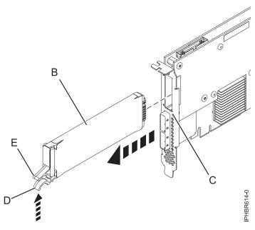
Figure 27. Replacing the 574E cache battery
