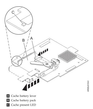
Figure 25. Removing the 57B7 cache battery
