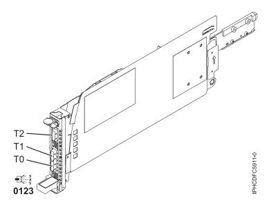
Figure 12. CCIN 57BA PCIe x8 Ext Dual-x4 3 Gb SAS adapter and cable card
