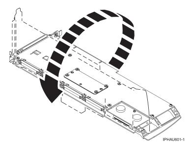
6. Remove four screws **B** from the removable cache card as shown.
