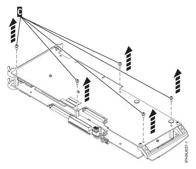
6. Carefully lift the 571F storage adapter off the standoffs and set it on the ESD protective surface.
