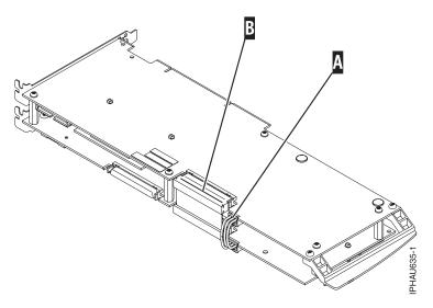
4. Disconnect battery cable **A** and SCSI cable B from the 571F storage adapter. Leave the other end of the cables attached to the 575B auxiliary cache adapter.
