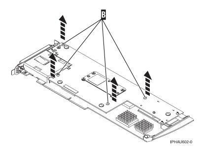
7. To separate the cards, turn the jack screw counterclockwise until you feel the cards separate.
