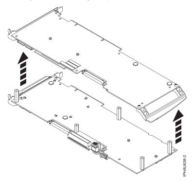
7. Turn the 571F storage adapter over so the components are facing up and locate the cache directory card **D** on the 571F storage adapter. It is the small rectangular card mounted on the I/O card.
