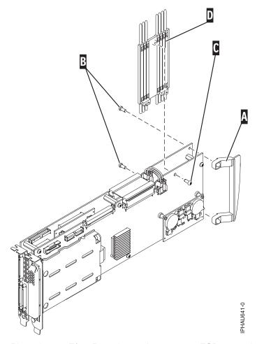
3. Place the 571F/575B card set adapter on an ESD protective surface and orient it as shown.
