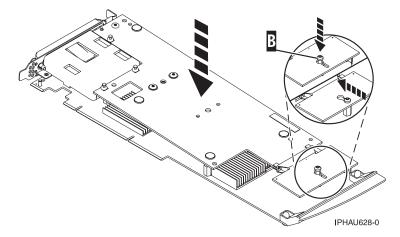
c. Press down on the area of the card over the connector to fully seat the connector.
