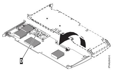
8. Unseat the connector on the cache directory card by wiggling the two corners that are farthest from the mounting pegs. To disengage the mounting pegs, pivot the cache directory card back over the mounting peg.
