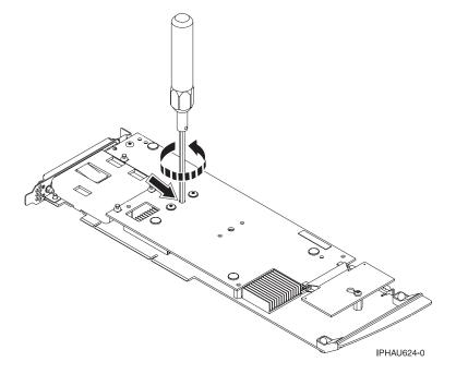
15. Carefully slide the removable cache card towards the plastic handle. Slightly lift up the back portion of the cache card freeing the cache directory card's keyhole slot from its retaining screw.
