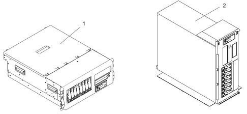
The 296/C3 is a 4 EIA-unit drawer designed to be housed in a 19-inch rack, while the 296/E3 is a deskside system. Both models can be configured as a 1-way to 2-way symmetric multiprocessing (SMP) system; each can have up to 8 hot-swapable disk drives and 6 hot-swapable PCI adapters. Both models support redundant hot-swappable power supplies and cooling fans.
