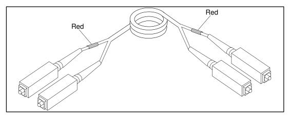
Figure 18. SC/SC Fiber Cable.
