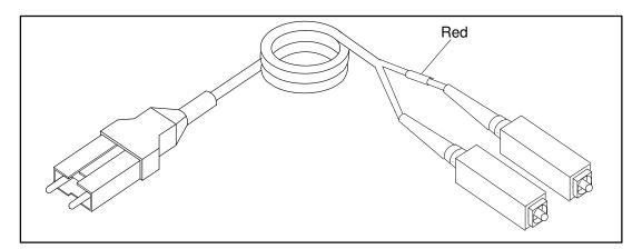
Figure 17. MIC/SC Fiber Cable.
