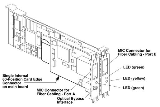
Figure 4. FDDI Fiber Dual Ring (Type B2-S MCA Adapter).
