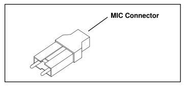
Figure 14. MIC Fiber Loopback Plug.
