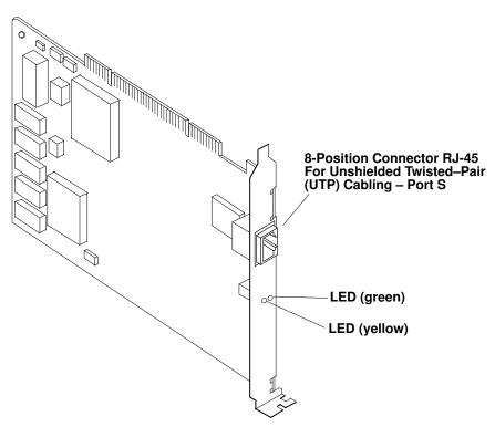
Figure 2. FDDI UTP Single Ring Adapter (Type B5-3 PCI).
