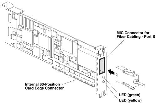
Figure 3. FDDI Fiber Single Ring (Type B2-R MCA Adapter).
