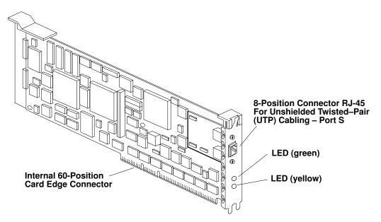
Figure 1. FDDI UTP Single Ring Adapter (Type B2-P MCA).
