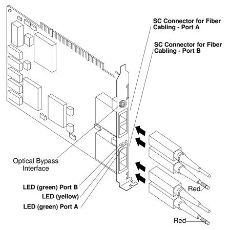
Figure 6. FDDI Fiber Dual Ring (Type B5-5 PCI Adapter).
