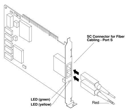
Figure 5. FDDI Fiber Single Ring (Type B5-4 PCI Adapter).
