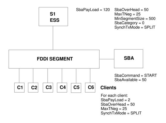
Figure 9. Static Mode Configuration – Example.
