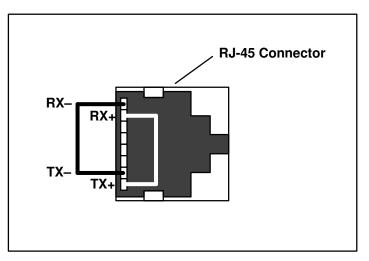
Figure 12. RJ-45 Pinout Showing Loopback.
