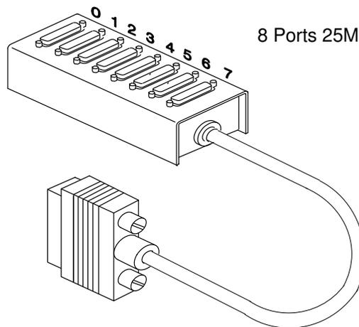
Figure 2. 8-Port DB-25 Connector Box
