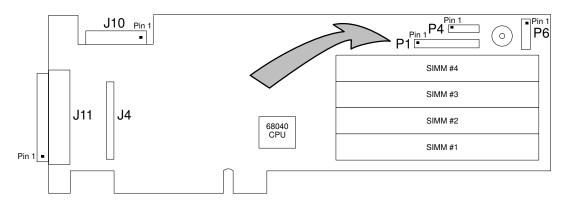
Figure 9. Installing Jumper on P1
