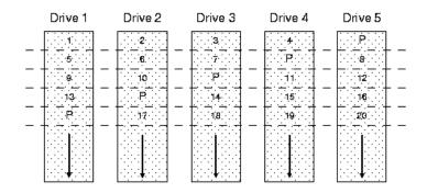
Figure 48. Data Redundancy - Rotating Parity
