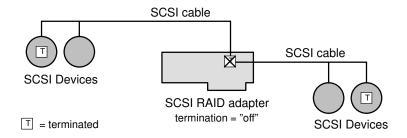
Figure 5. SCSI Two-Cable Termination
