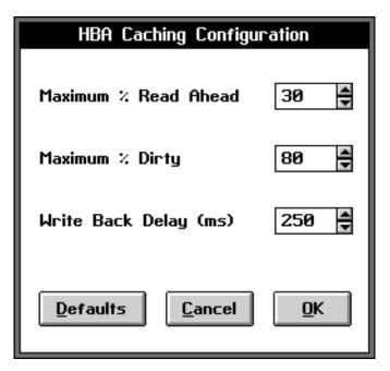
Figure 16. HBA Caching Configuration Window for B4-4 adapter
