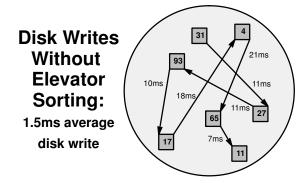
Figure 37. Disk Writes Without Elevator Sorting
