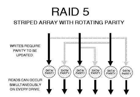
Figure 47. Striped Array with Rotating Parity
