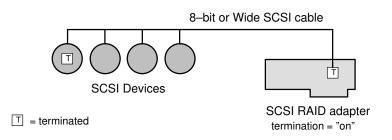
Figure 3. SCSI Single Cable End Termination
