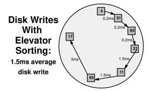
Figure 36. Disk Writes With Elevator Sorting
