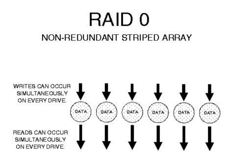
Figure 42. Non-redundant Striped Array
