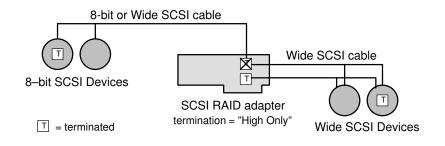
Figure 6. SCSI 8-bit/Wide Cables Termination
