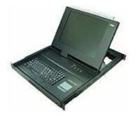
Figure 24. Integrated console example
