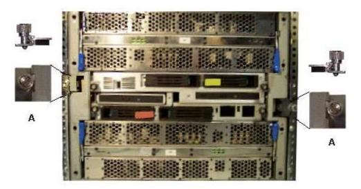
Figure 4. Installing front stoppers
