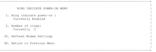
Ring indicate is enabled by default on both serial port 1 (S1) and serial port 2 (S2). When ring indicate power on is enabled, call-in is disabled.
