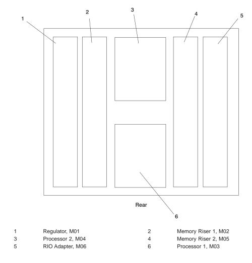
**Note:** In order for the system to boot, the first processor card slot (M03) must be populated.
