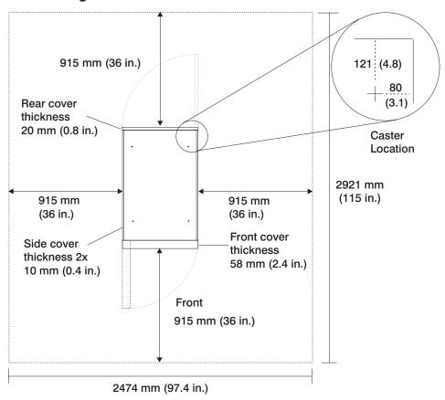
**Note:** Rack units are large and heavy and are not easily moved. Because maintenance activities require access at both the front and back, allow for extra room. The footprint shows the radius of the swinging doors on the I/O rack. The figure shows the minimum space required.
