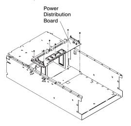
14. Remove the power distribution board.
