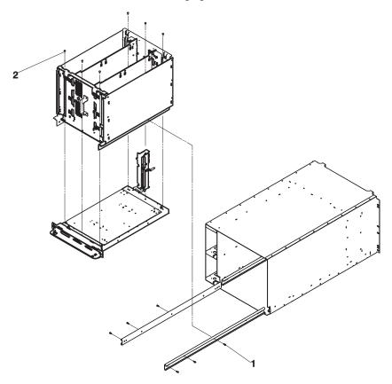
16. Place the CEC card-cage on a suitable work surface.
