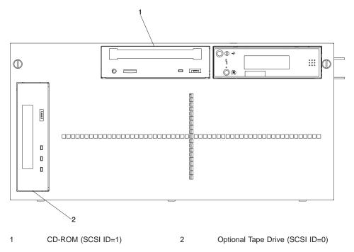
**Note:** The SCSI IDs shown for the media indicate how installed devices are set when shipped from the factory.
