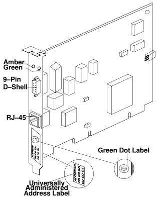
Figure 3. Type B5–R Token Ring PCI Adapter
