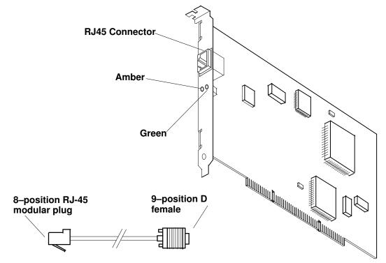
Figure 1. Type 8-T Token Ring PCI Adapter and associated Conversion cable
