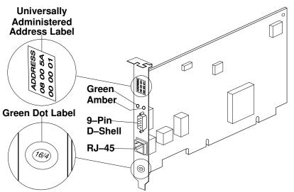
Figure 2. Type B5–J Token Ring PCI Adapter
