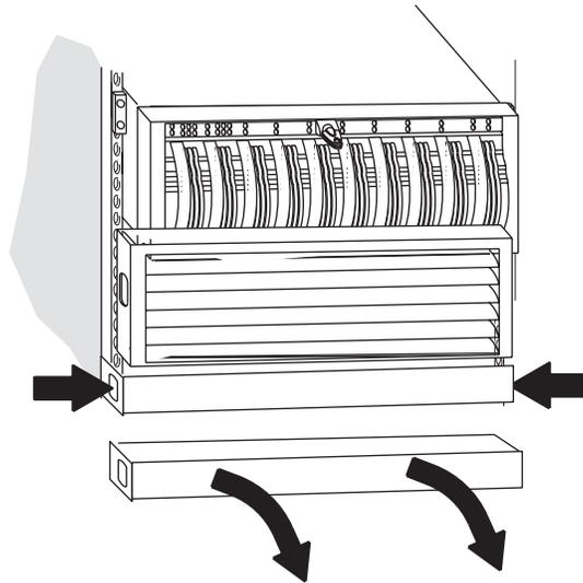
5. Remove the two screws that fasten the front of the target SPS to the mounting tray as shown below.
