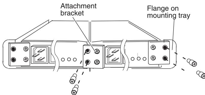
5. Working from the front of the tray, fasten two screws through the front panel into each SPS as shown below.
