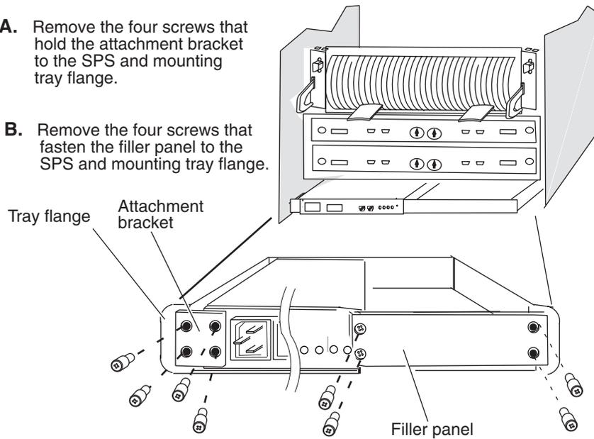
8. Remove the SPS you want to service or replace. Removal of the left SPS is shown below.
