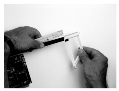
d. Ensure that the adjustable top retainer clip catches the corner of the adapter as shown in the following figures.
