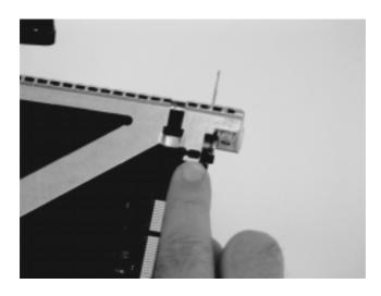
iii. Turn the cassette assembly over so the cover is up and check the cover latch to ensure it is holding the bezel to the cover as shown.
