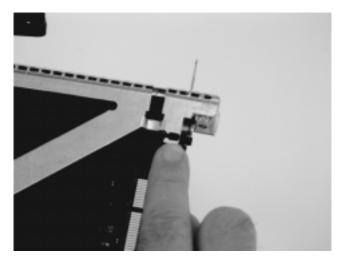
iii. Align the top of the bezel assembly into the grooves on the top of the cassette assembly and then push the bezel onto the cassette linkage until the tab on the top of the bezel is seated in the recess of the cassette assembly.
