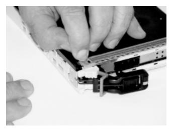
m. Insert the bushing lock pin into the hole in the bushing. Push on the pin until it seats.
