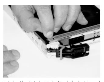
m. Insert the bushing lock pin into the hole in the bushing and push it in until it seats.
