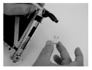
i. Ensure that the shield slides up inside the top of the cassette.
