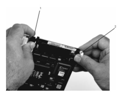
1 Long Adapter Arm Adjustable Retaining Clip
