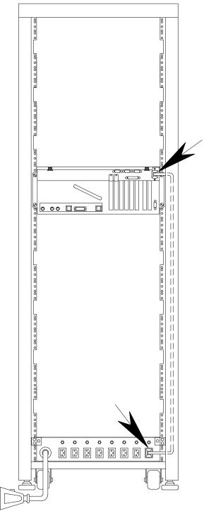
c. Set the circuit-breaker related to the chosen PDU outlet to ON.
