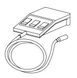
Connect the keyboard to the dedicated connector at the rear of the CPU drawer. Do not force the cable plug into the socket.
