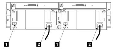
Figure 24. Removing the Power from a 2104 Model DU3
