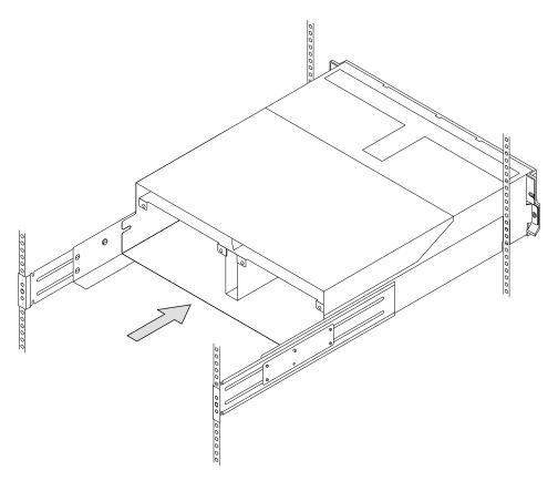
Figure 51. Pushing the Frame Assembly Forward
