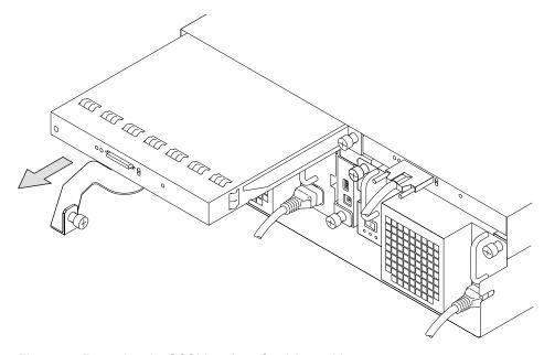
Figure 45. Removing the SCSI Interface Card Assembly
