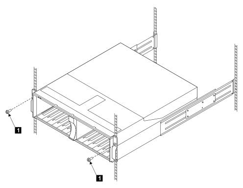
Figure 55. Removing the Front Mounting Screws
