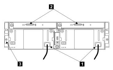
Figure 16. Power Cables and SCSI Connectors (2104 Model DU3)
