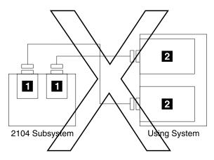
Figure 72. Two Adapters in One Using System Connected to One 2104 (Single-Bus Mode). **This configuration is not valid.**
