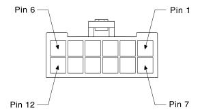
Figure 11. Mainline-Power Connector (-48 V dc)
