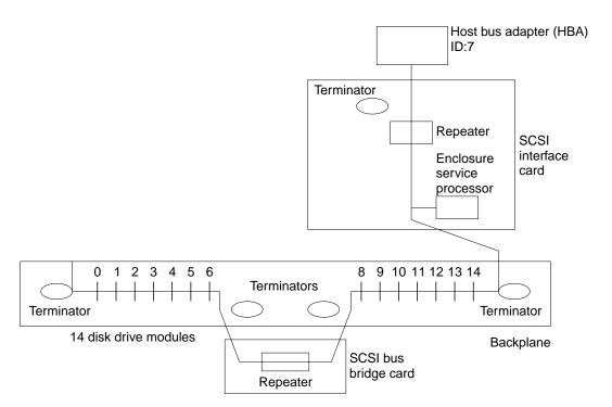
Figure 13. Single Bus, One SCSI Attachment, 14 Disk Drive Modules
