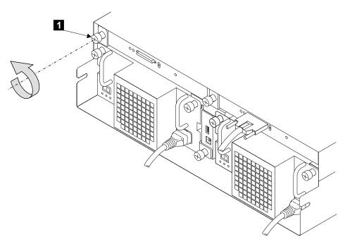
Figure 43. Unscrewing the Thumbscrew
