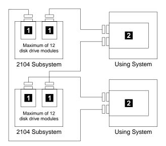
Figure 63. One Adapter in Each of Two Using Systems Connected to Two 2104s (Single-Bus Mode)
