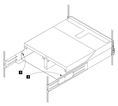
Figure 50. Loosening the Back Mounting Screws
