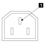
Figure 17. Ground Pin (2104 Model DU3; 220 V)
