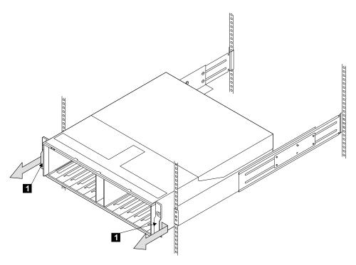
Figure 52. Removing the Frame Assembly from the Rack
