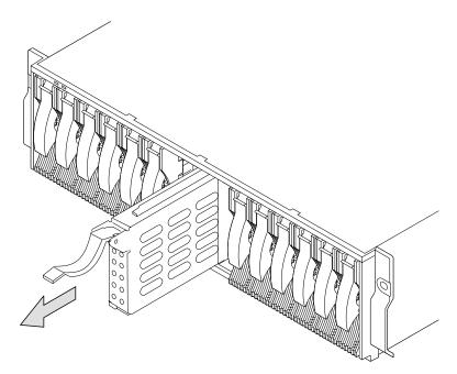
Figure 34. Removing the SCSI Bridge Card Assembly
