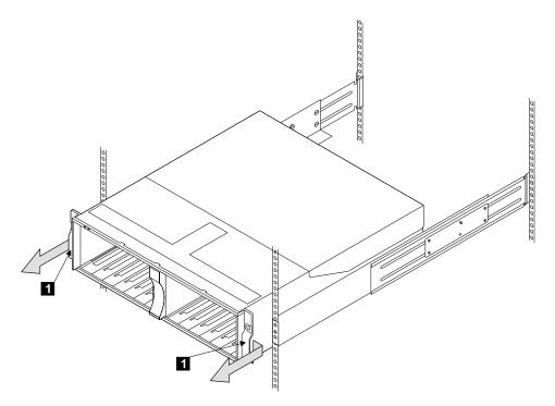
Figure 58. Removing the 2104 Model DU3 from the Rack
