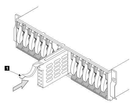
Figure 35. Installing the SCSI Bridge Card Assembly
