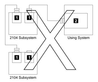
Figure 73. One Adapter in One Using System Connected to Two 2104s via the SCSI Interface Card Assemblies. This configuration is not valid.
