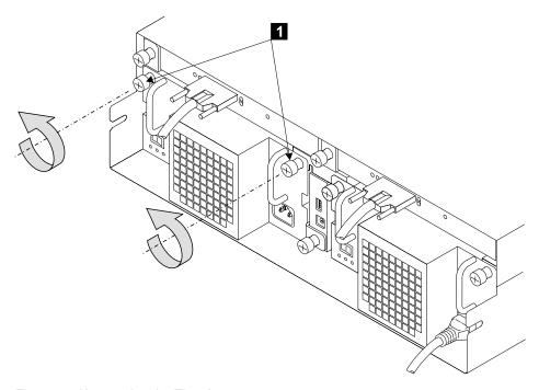
Figure 38. Unscrewing the Thumbscrews
