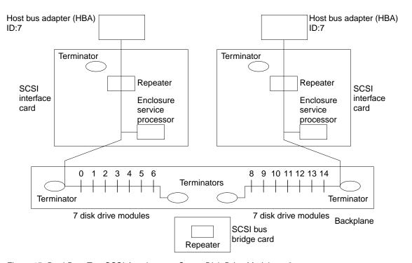
Figure 15. Dual Bus, Two SCSI Attachments, Seven Disk Drive Modules x 2
