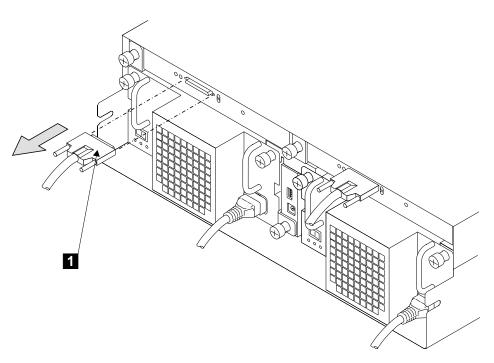
Figure 42. Disconnecting the SCSI Cable
