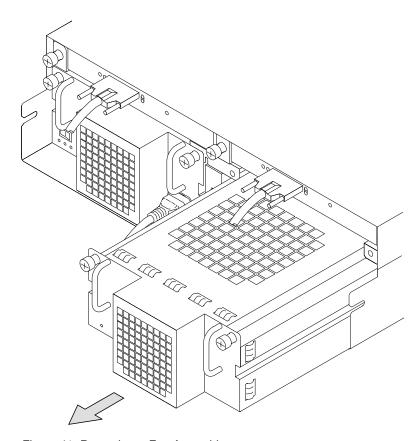
Figure 41. Removing a Fan Assembly
