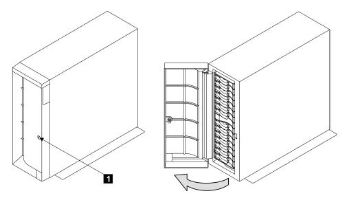
Figure 21. Opening the Front Cover of a 2104 Model TU3
