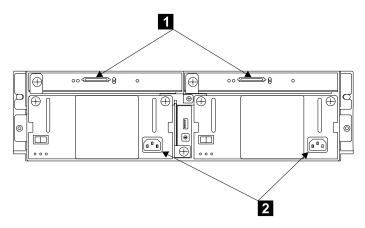
Figure 8. Back Connectors of the 2104 Model DU3
