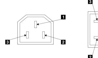
Figure 10. Mainline-Power Connector (220 V ac). The diagram shows the connector for a Model DL1 (left), and for a Model TL1 (right).
