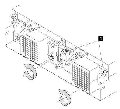
Figure 40. Unscrewing the Thumbscrews
