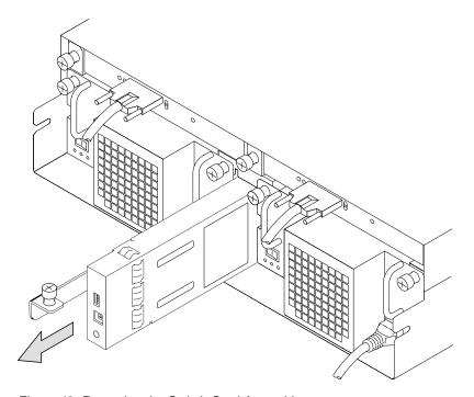
Figure 48. Removing the Switch Card Assembly
