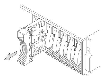
Figure 26. Removing a Dummy Disk Drive Module
