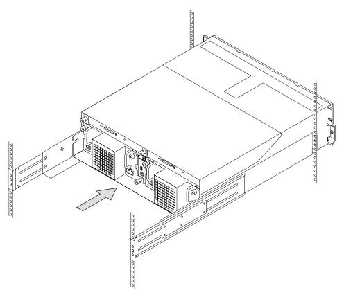
Figure 57. Pushing the 2104 Model DU3 Forward
