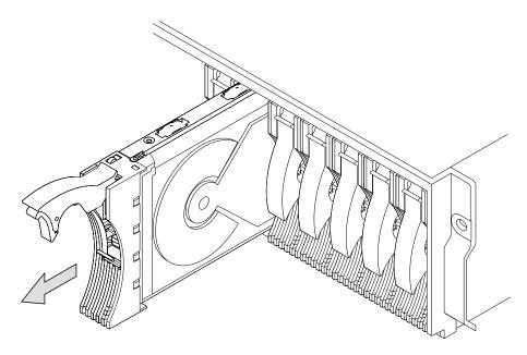
Figure 28. Removing a Disk Drive Module
