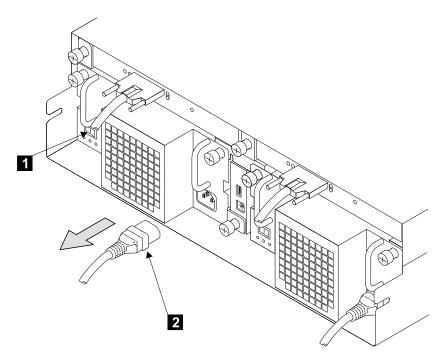
Figure 37. Switching Off and Disconnecting a Fan-and-Power-Supply Assembly
