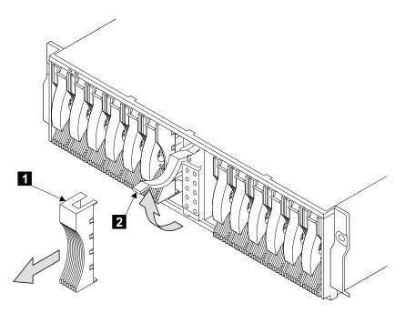
Figure 33. Removing the SCSI Bridge Card Assembly Cover
