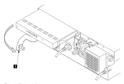
Figure 44. Opening the Lever
