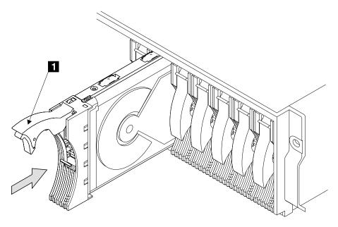
Figure 31. Installing a Disk Drive Module
