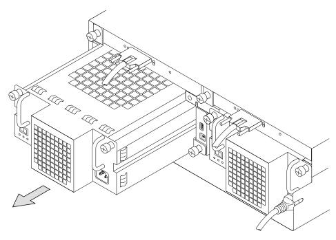
Figure 39. Removing a Fan-and-Power-Supply Assembly
