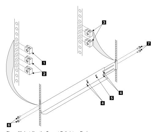
Figure 60. Installing the Support Rails into a Rack
