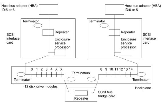
Figure 14. Single Bus, Two SCSI Attachments, 12 Disk Drive Modules
