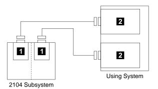
Figure 67. Two Adapters in One Non-HACMP Using System Connected to One 2104 (Dual-Bus Mode)
