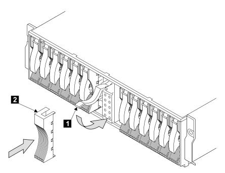
Figure 36. Closing the Handle and Installing the Cover
