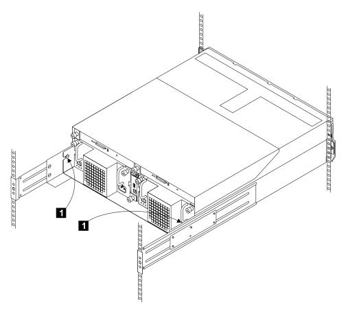
Figure 56. Loosening the Back Mounting Screws
