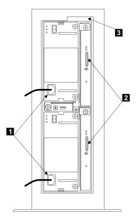
Figure 19. Power Cables and SCSI Connectors (2104 Model TU3)
