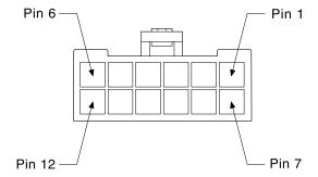
Figure 18. Ground Pins (2104 Model DU3: -48 V)
