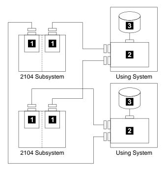
Figure 71. One RAID Adapter in Each of Two Non-HACMP Using Systems Connected to Two 2104s and an Internal RAID Array (Dual-Bus Mode)
