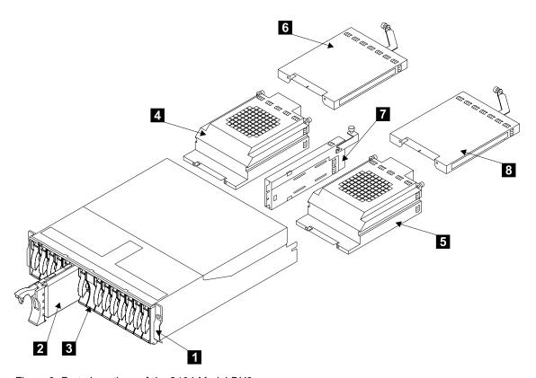
Figure 6. Parts Locations of the 2104 Model DU3
