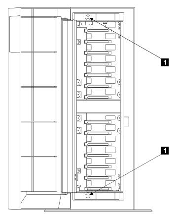
Figure 53. Removing the Frame from a 2104 Model TU3 (1)
