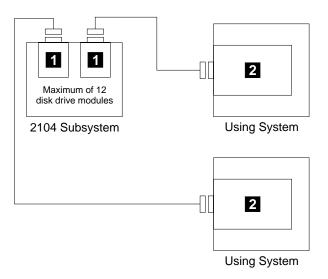
Figure 66. One Adapter in Each of Two Using Systems Connected to One (Single-Bus Mode)
