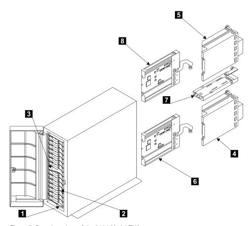
Figure 7. Parts Locations of the 2104 Model TU3
