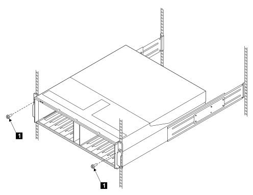
Figure 49. Removing the Front Mounting Screws
