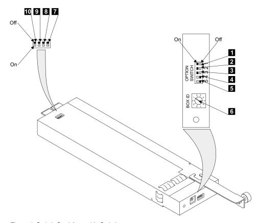
Figure 4. Switch Card Assembly Switches
