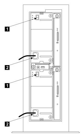
Figure 25. Removing Power from a 2104 Model TU3
