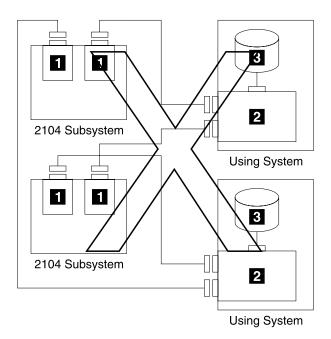
Figure 77. One RAID Adapter in Each of Two Using Systems Connected to Two 2104s. This configuration is not valid.
