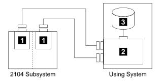
Figure 69. One Adapter in One Non-HACMP Using System Connected to One 2104 and an Internal RAID Array (Dual-Bus Mode)
