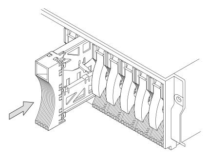
Figure 30. Installing a Dummy Disk Drive Module
