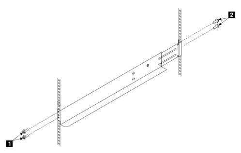
Figure 59. Removing the Support Rails from the Rack
